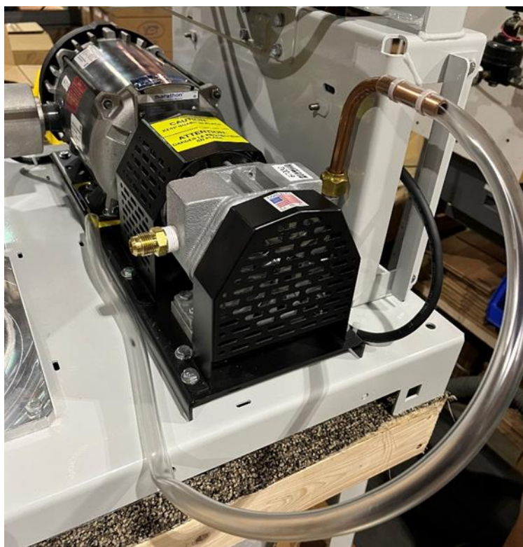
Figure 9-22: Vacuum Pump with the Blowout tube
