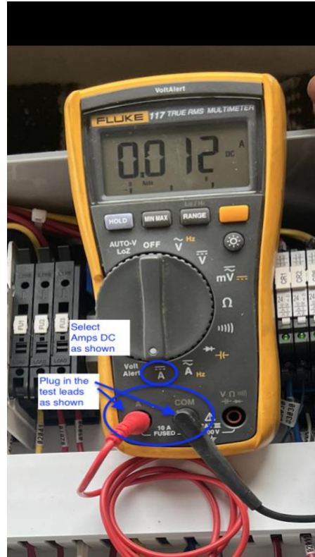
Figure 8-14: Example with Fluke multimeter set-up to measure 4-20 mA DC current
