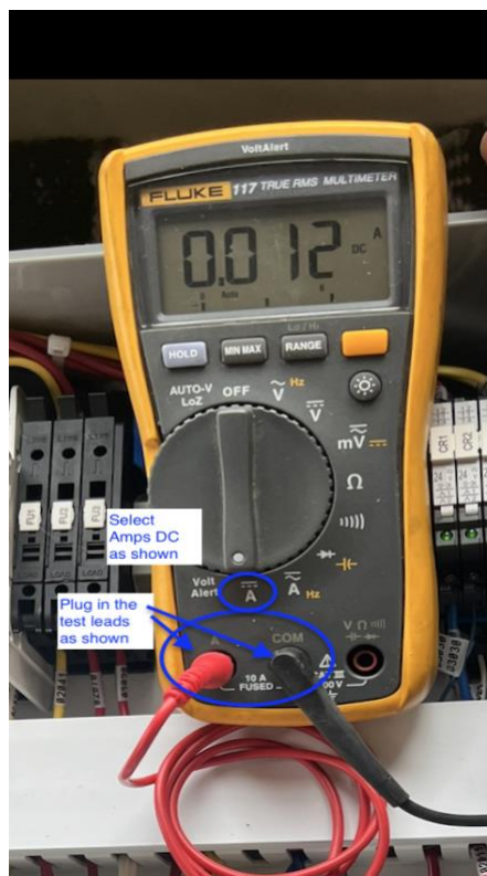
Figure 8-14: Example with Fluke multimeter set-up to measure 4-20 mA DC current
