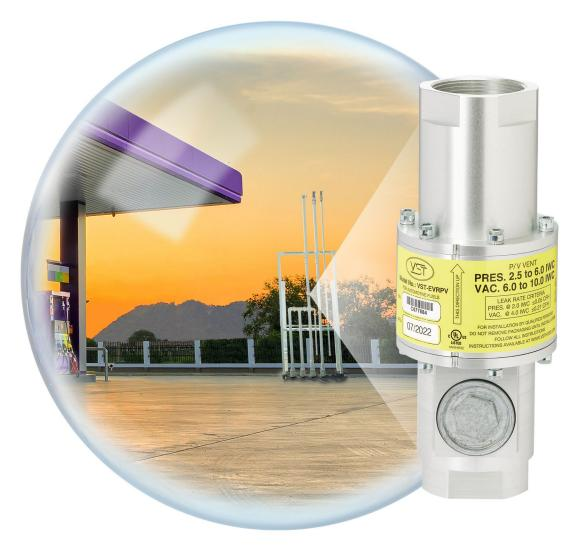
**VST SENTRY**<sup>™</sup> **Pressure Vacuum (P/V) Valves** are highly engineered products designed to protect the structural integrity of the Underground Storage Tank (UST) from extreme positive and negative pressure conditions caused by fuel drops and vehicle dispensing. These robustly, unique P/V valves help to prevent unwanted vapor emissions from escaping into the environment.
