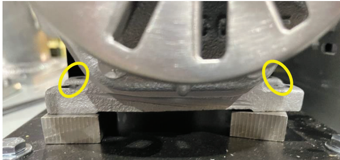
Figure 7-10: Vacuum Pump Mounting Bolts
