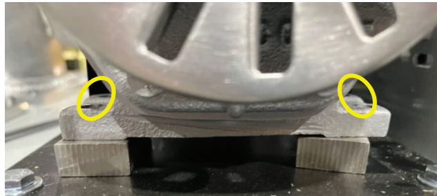
Figure 9-8: Vacuum Pump Mounting Bolts
