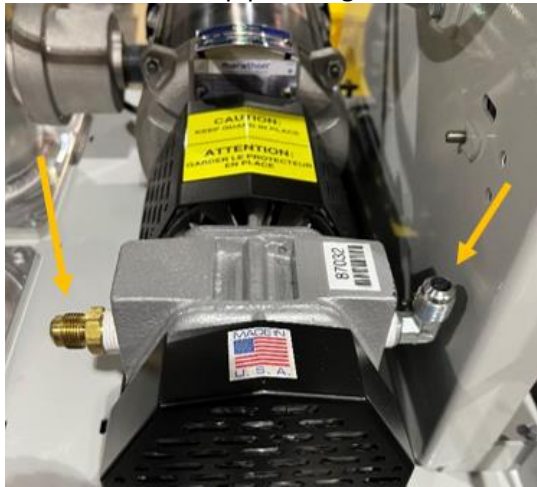
Figure 9-14: Two Tubes Removed from Vacuum Pump
