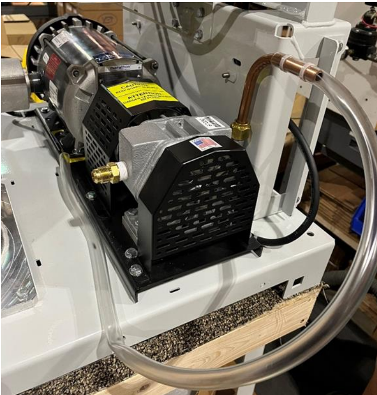
Figure 9-22: Vacuum Pump with the Blowout tube
