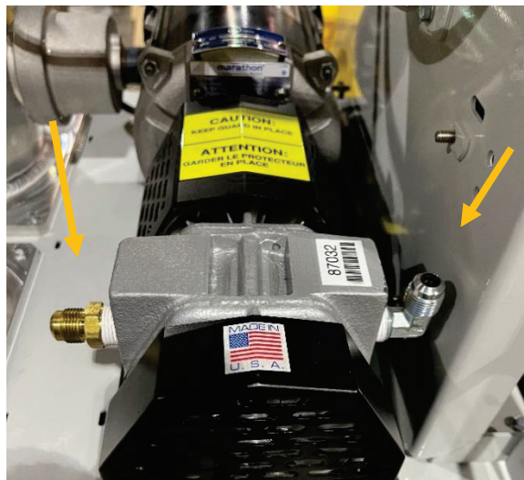
Figure 7-8: Two tubes removed from vacuum pump
