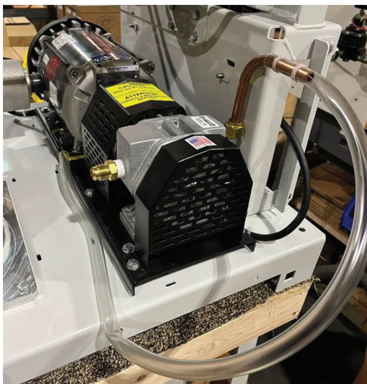
Figure 9-22: Vacuum Pump with the Blowout tube
