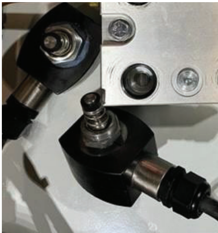
Figure 9-21: Solenoids with the Core Assembly Inside
