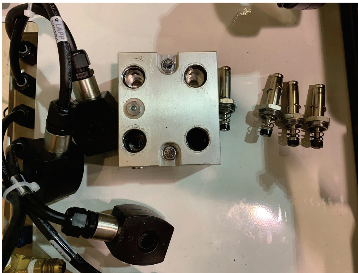
Figure 9-20: Solenoids Arranged Out of the Way
