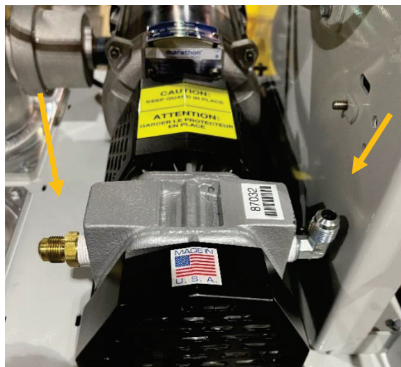
Figure 9-6: Two tubes removed from vacuum pump
