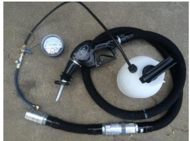
Separated breakaway half with a hole drilled and tapped in the side.
