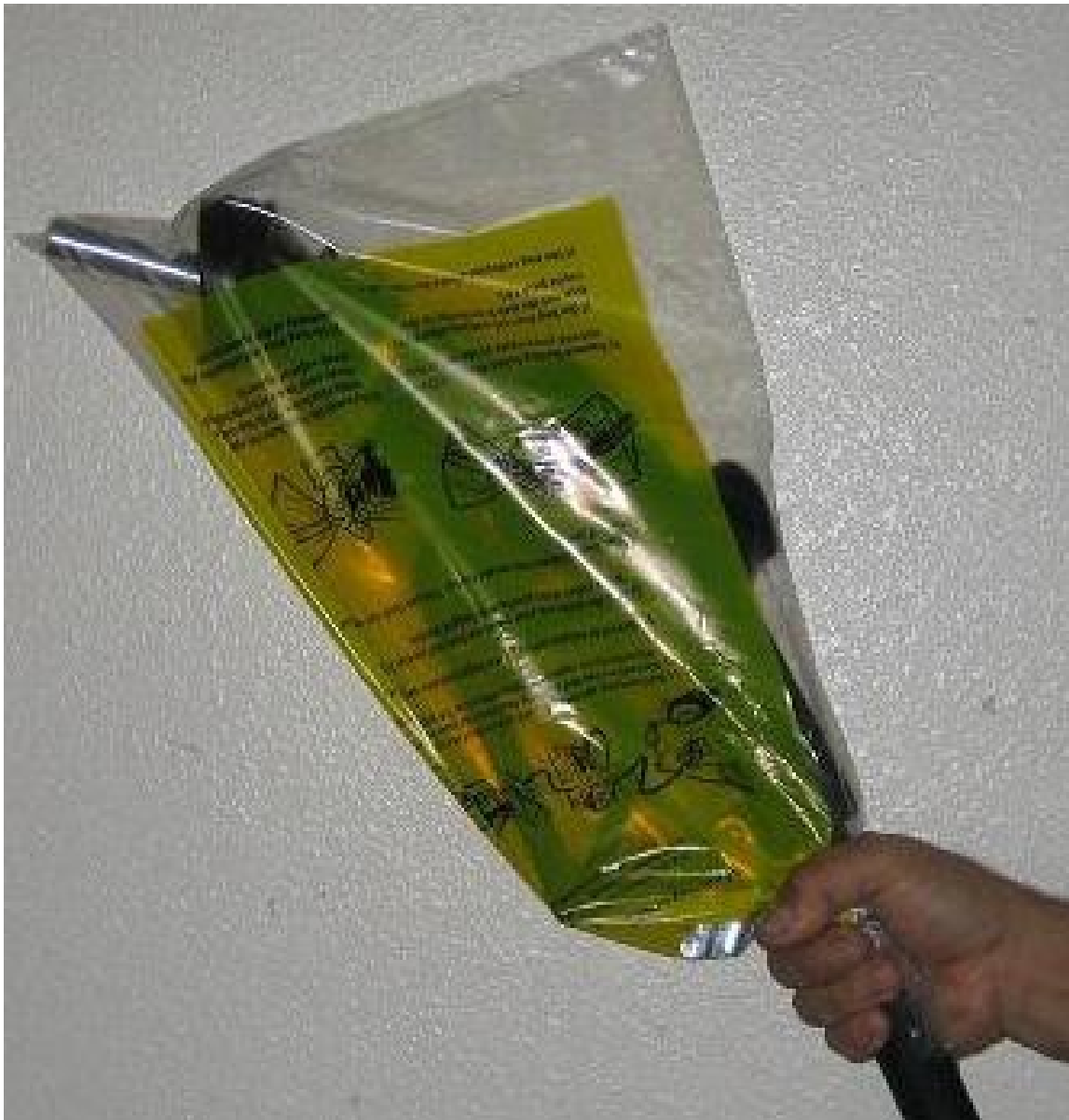
FIGURE 7-1 Typical Example of Bagging a Nozzle
