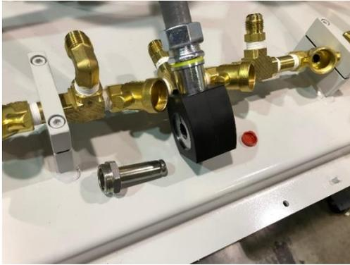
Figure 9-27: Solenoid with Solenoid Base and RED Cap
