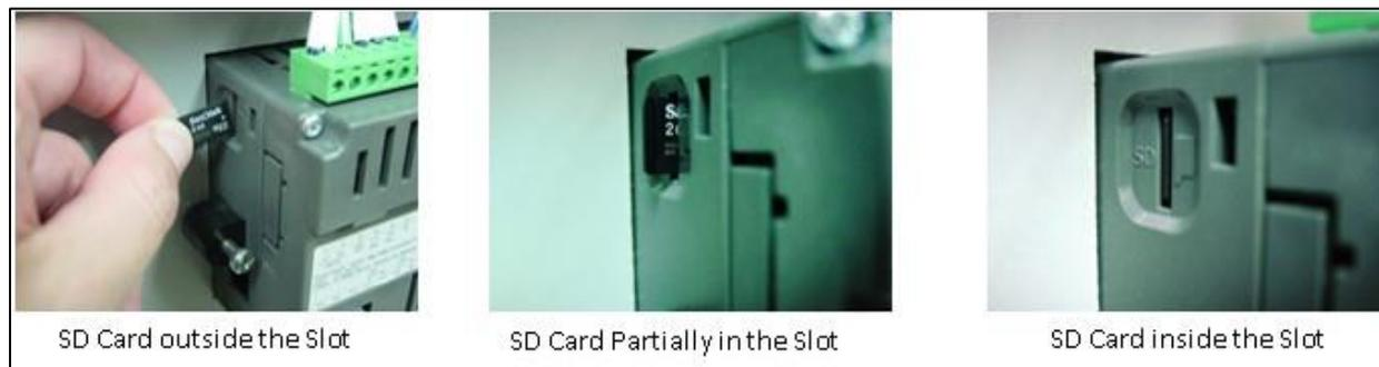
Figure 11-6: Inserting and Removing the SD Card from the PLC
