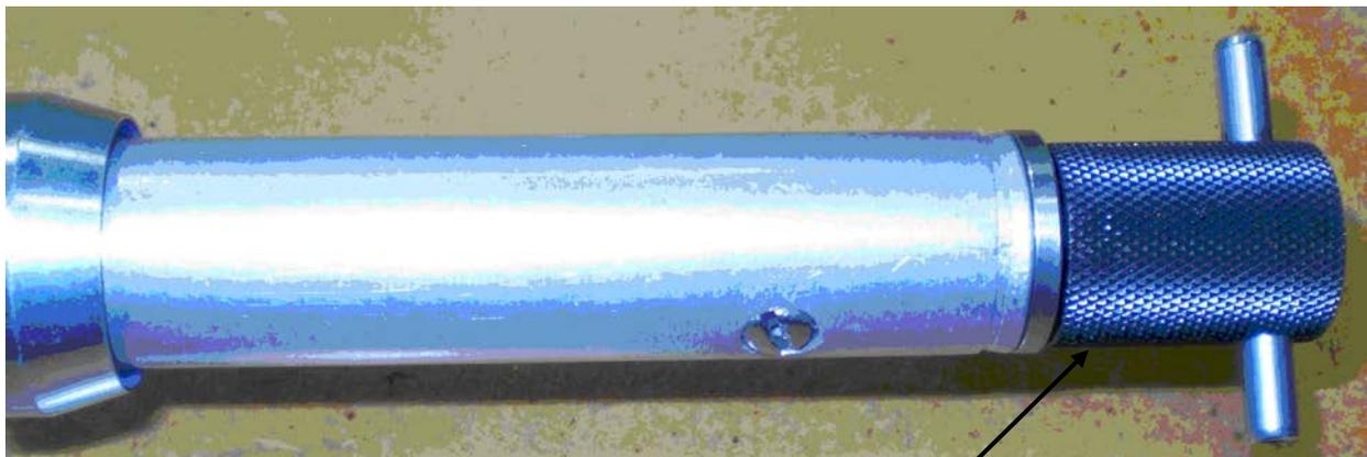
**Plug properly inserted into nozzle spout.**
