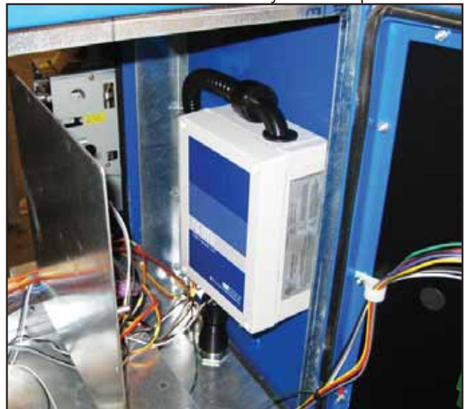
Figure 15: DTU Attached to Dispenser
