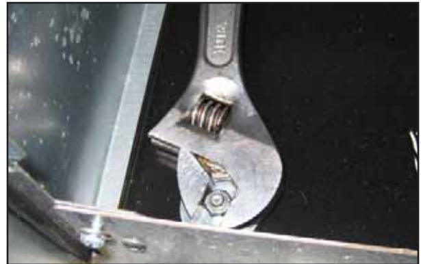
Figure 4: Remove Hole Plug
