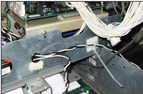
Figure 12: Attach Power Wiring Harness
