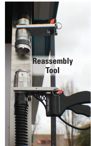
Figure 4: Attach Reassembly Tool
