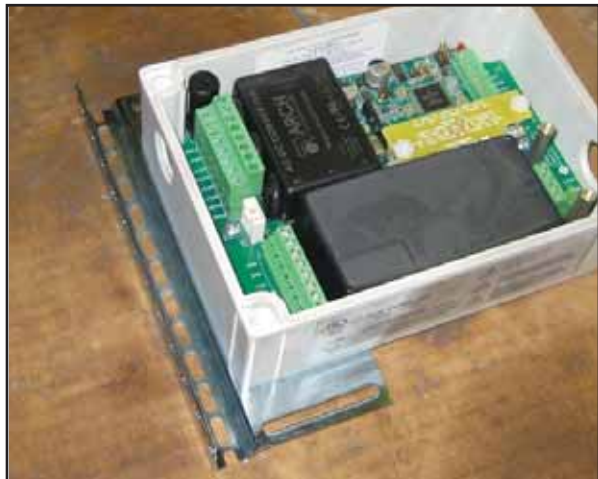
Figure 7: Mounting Bracket on DTU
