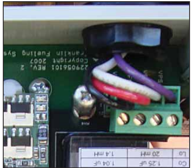
Figure 12: Wiring Connection to DTU
