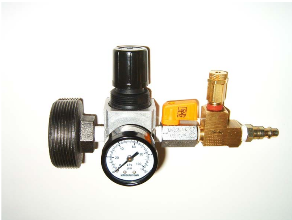
Figure 20: Typical Leak Check Test Fixture
