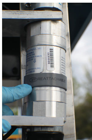
Figure 8: Reposition Retaining Sleeve
