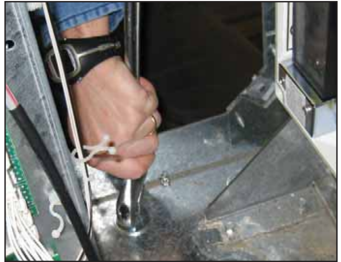
Figure 8: Remove Hole Plug
