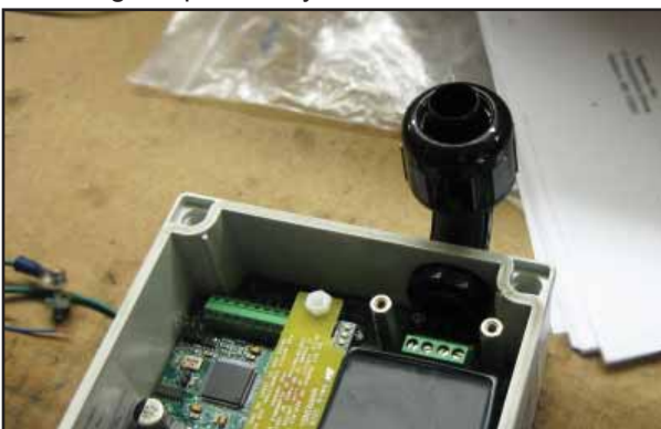
Figure 7: 90-Degree Fitting Installed
