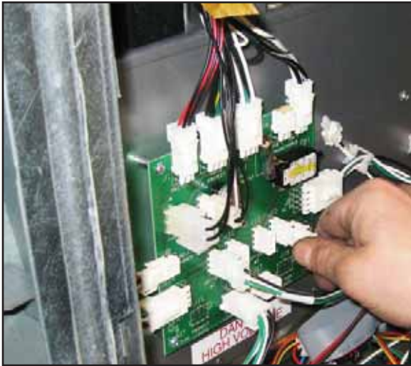
Figure 17: Attach White Connector
