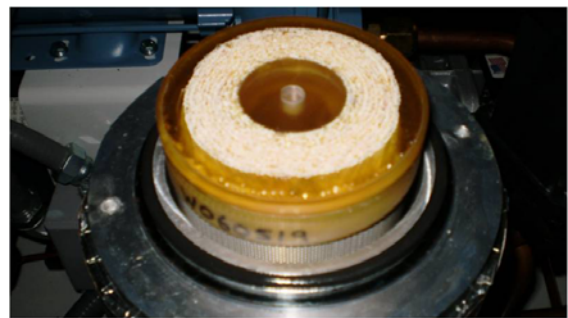
Figure 30: Exposed membrane with top plate removed.
