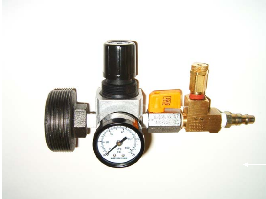
Figure 7: Typical Leak Check Test Fixture
