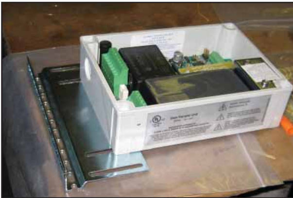
Figure 2: Install Mounting Bracket
