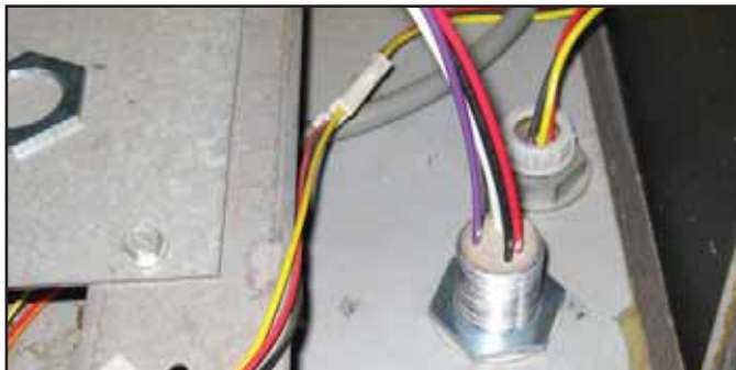
Figure 7: Potted Nipple Assembly Attached
