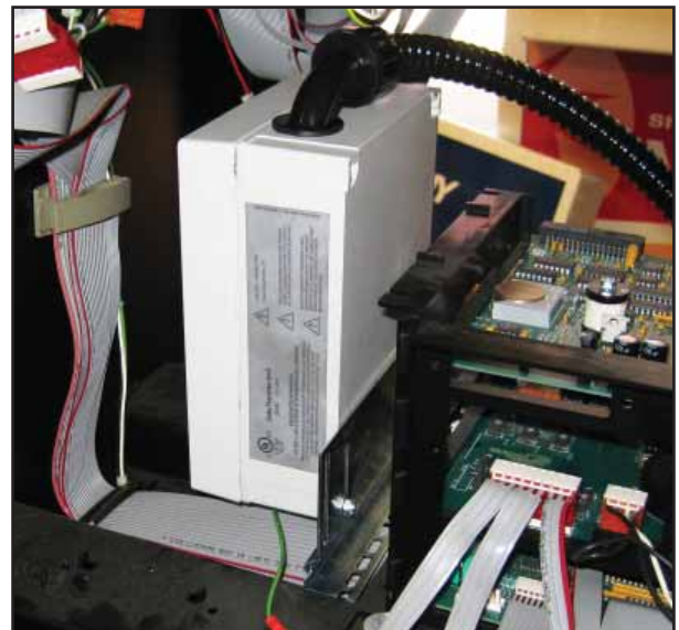
Figure 15: Attach DTU Mounting Bracket
