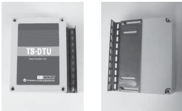
Figure 5: Mounting Bracket On Side Of Unit
