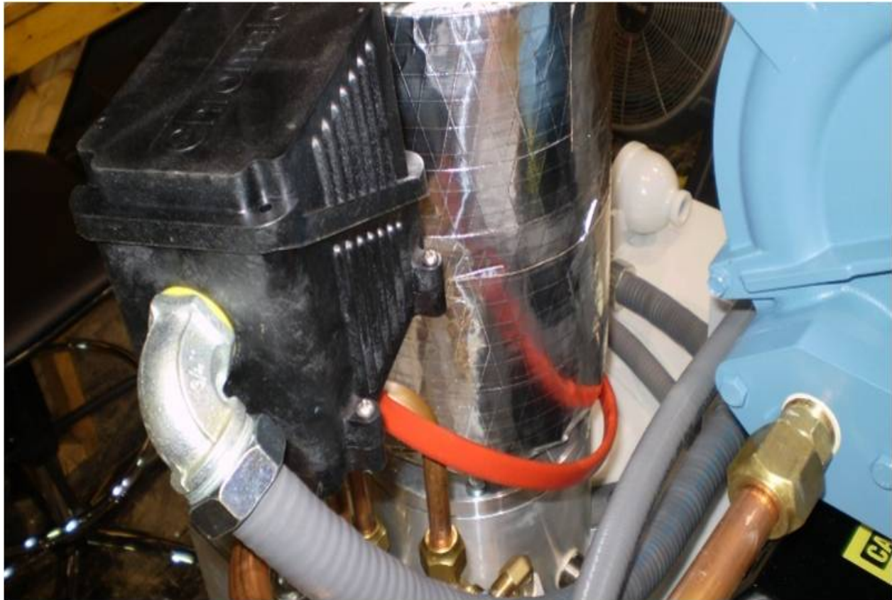
Figure 48: Installed electrical junction box with electrical connections
