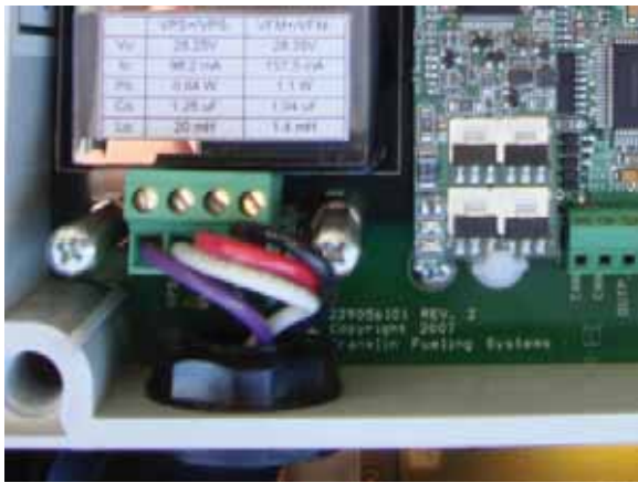
Figure 15: Wires Connected to DTU
