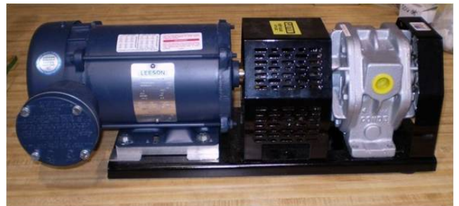
Figure 34: Vacuum and motor assembly
