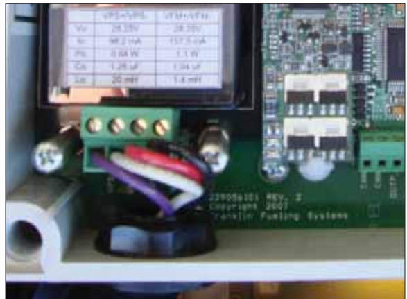
Figure 13: Wires attached to DTU
