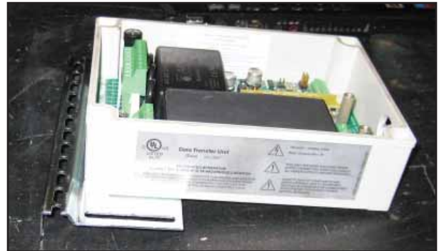
Figure 10: Mounting Bracket on DTU
