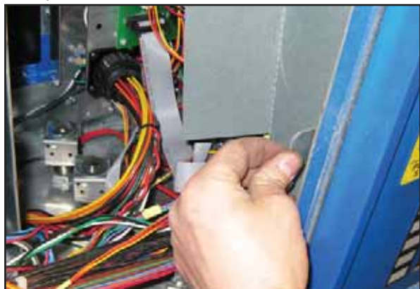
Figure 2: Release Inside Latch
