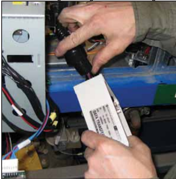
Figure 12: Pull wires through 90-degree fitting
