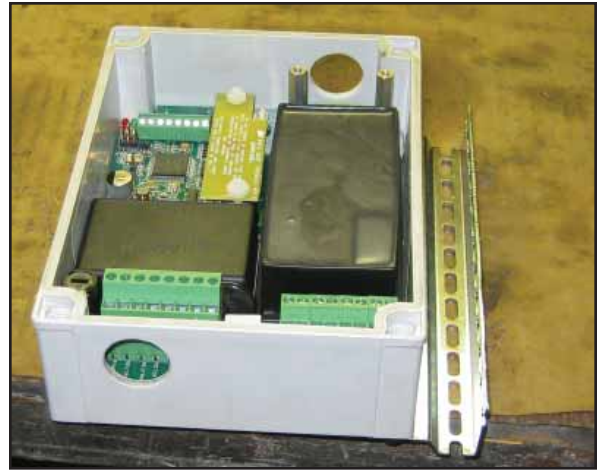
Figure 7: DTU Mounting Bracket Installed
