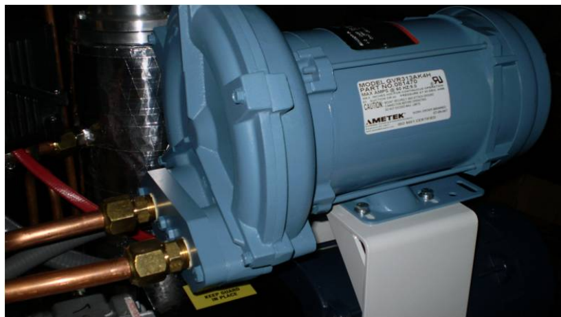
Figure 24: Blower inlet and outlet tubing connections and mounting bolts
