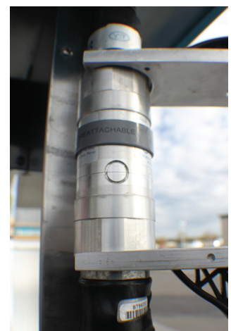
Figure 5: Align Poppet Pin from upper to lower half of breakaway and finish alignment
