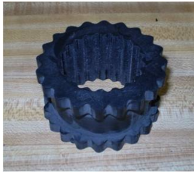
Figure 36: Drive coupling rubber insert
