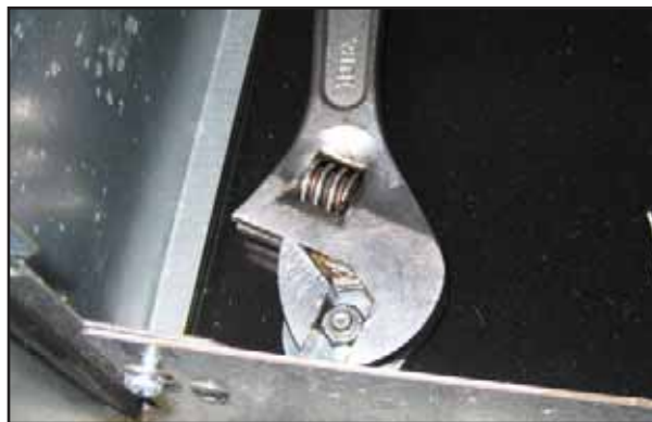
Figure 3: Remove Hole Plug
