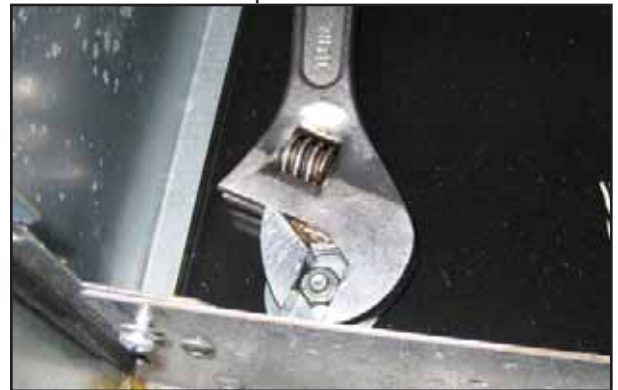
Figure 4: Removing Hole Plug
