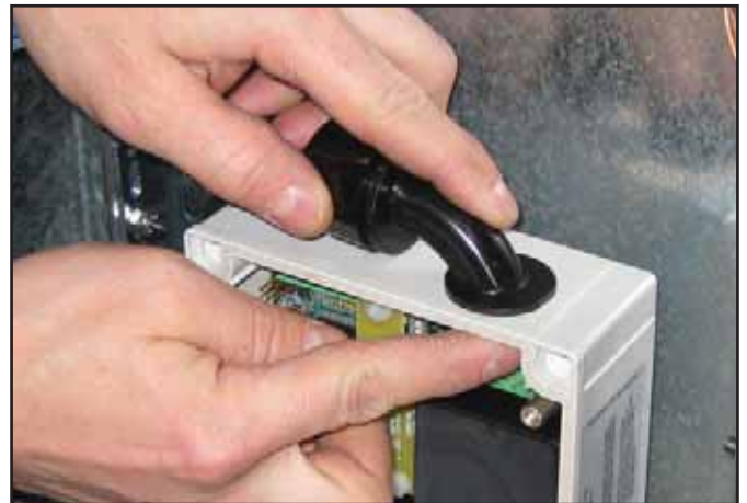
Figure 13: Attach 90-Degree Fitting
