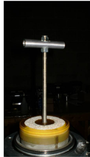
Figure 31: Membrane extraction tool
