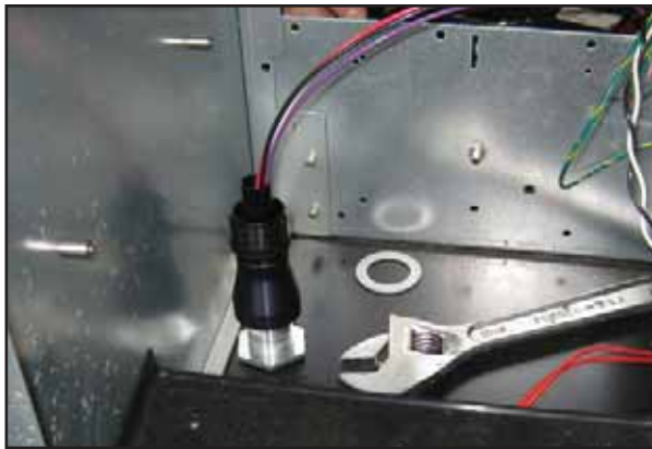
Figure 5: Straight Conduit Installed
