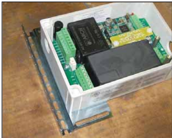
Figure 6: Mounting Bracket on DTU
