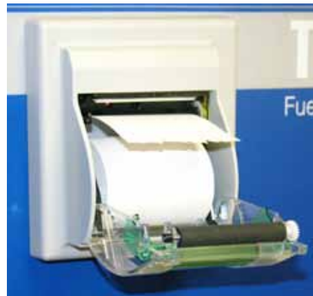
Figure 9: Paper Loaded Correctly
