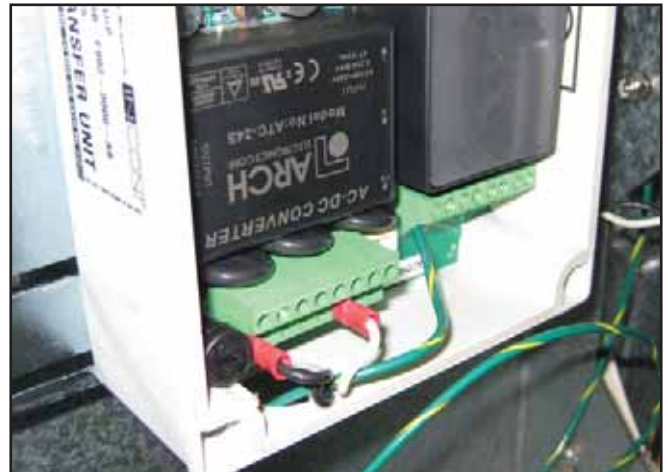
Figure 4: Attach Power Wiring
