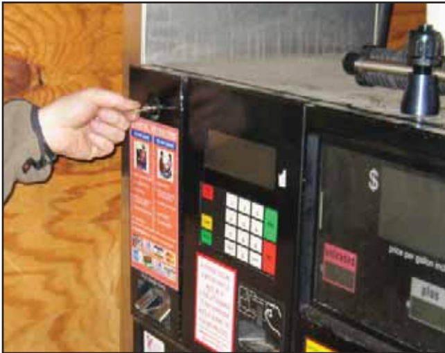
Figure 2: Unlock Printer Door
