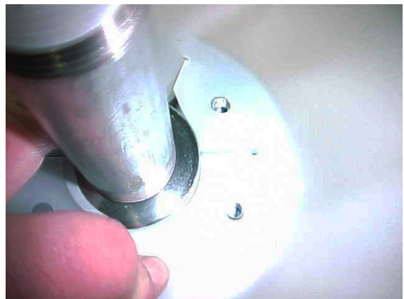
Figure 2: Place Bladder on Flange
