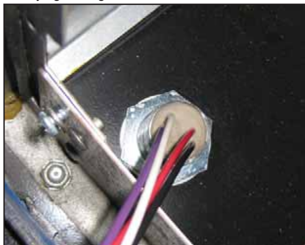
Figure 4: Potted Nipple Installed
