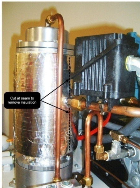
Figure 38: Seam to cut to remove the insulation
