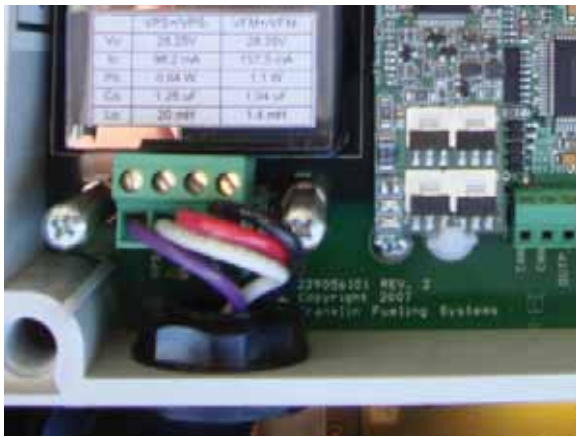
Figure 16: Wires Connected to DTU
