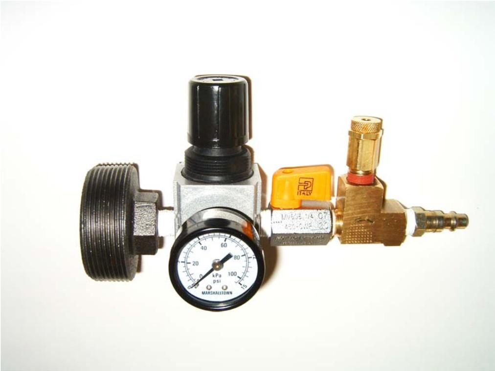
Figure 20: Typical Leak Check Test Fixture
