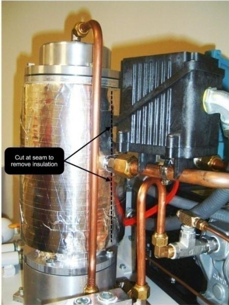
Figure 38: Seam to cut to remove the insulation
