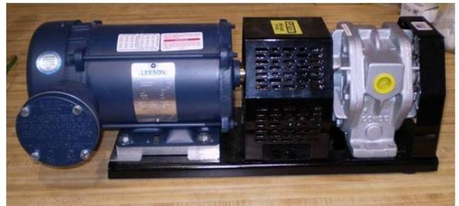
Figure 34: Vacuum and motor assembly
