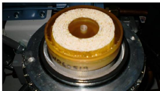
Figure 30: Exposed membrane with top plate removed.
