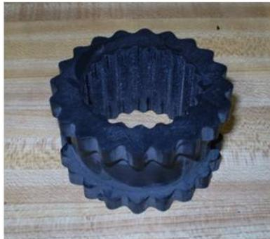
*Figure 36: Drive coupling rubber insert*
