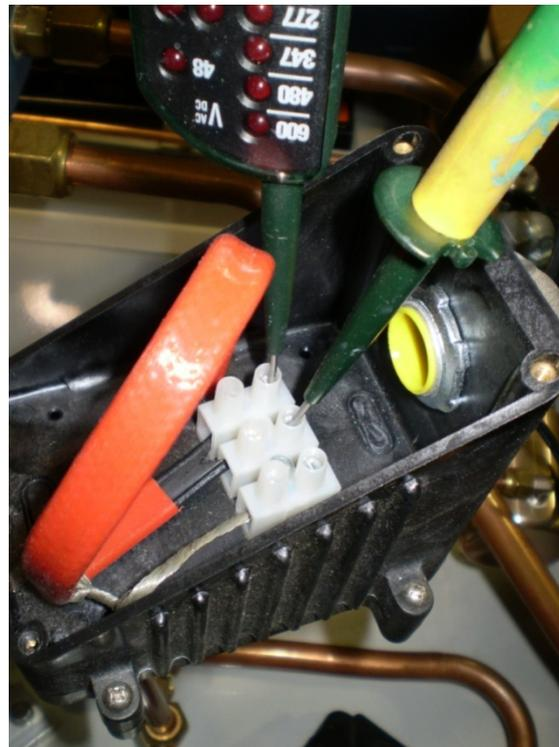
Figure 16: Heat Trace Circuit Test
