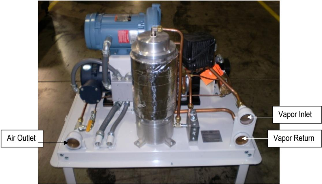
Figure 19: Processor Inlets & Outlets
