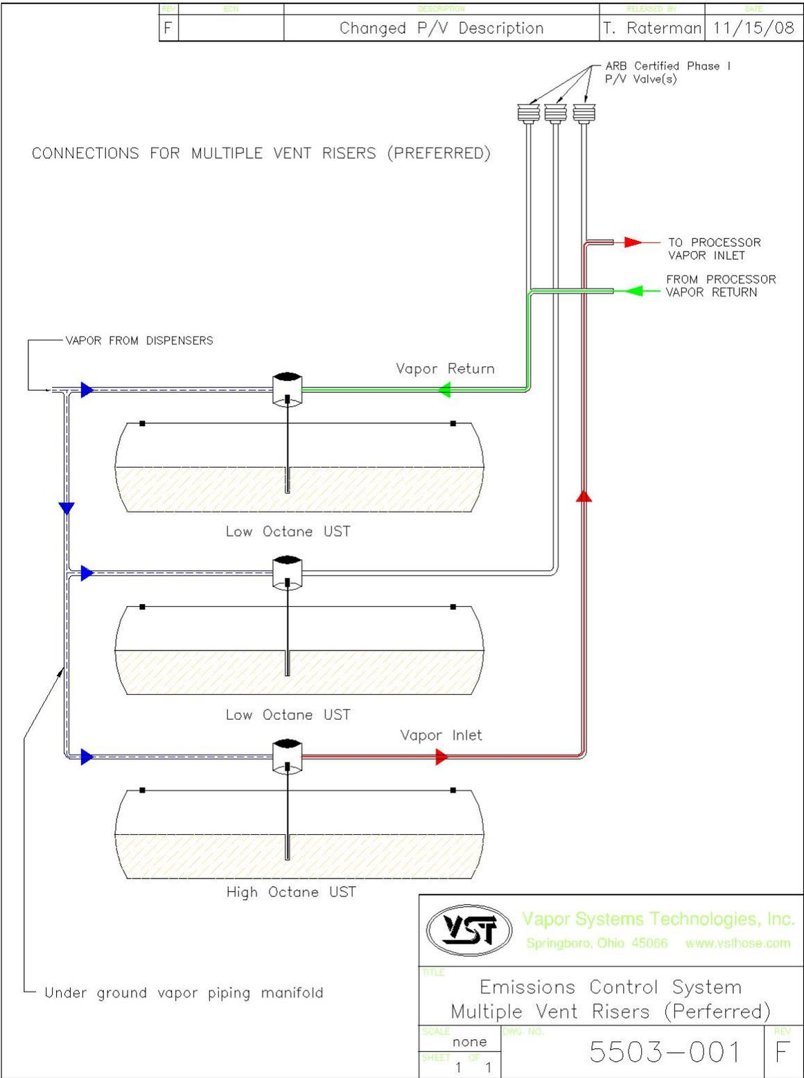
Figure 11: Processor Connections with Multiple Vent Risers
