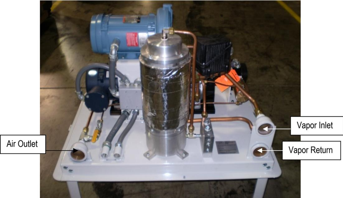
Figure 6: Processor Inlets & Outlets
