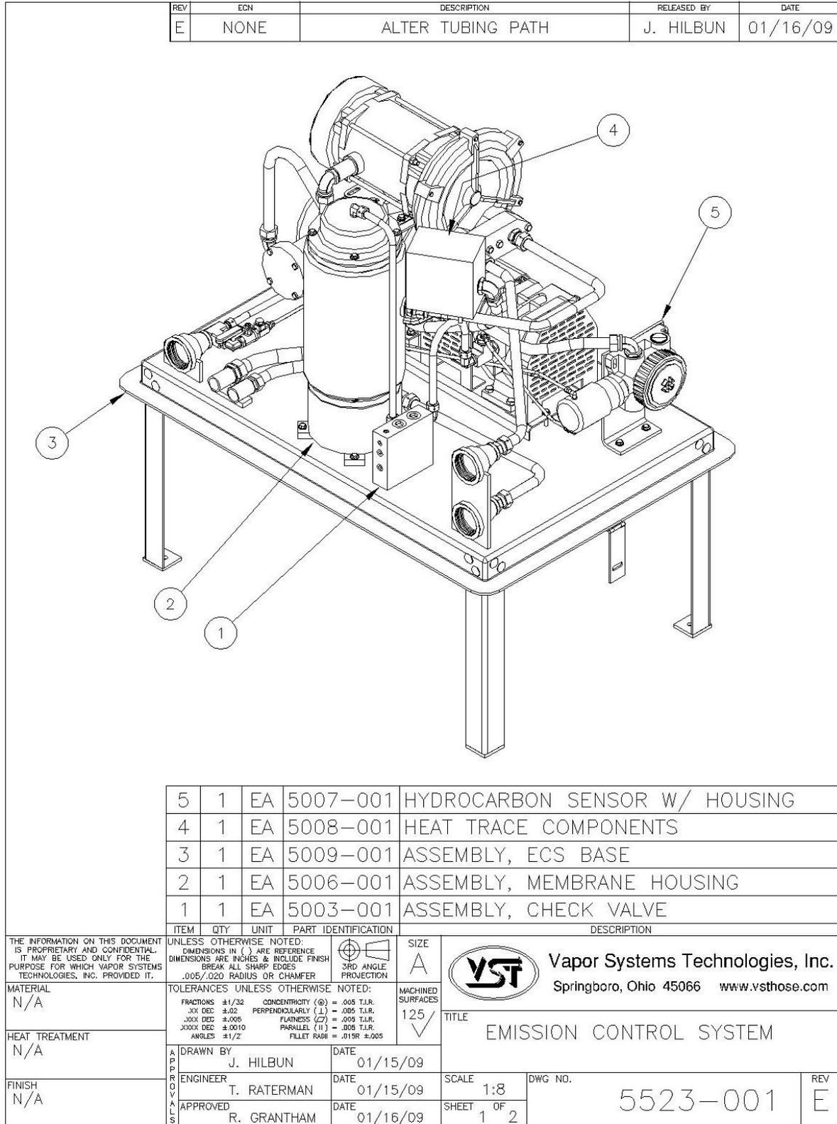
Figure 4: Processor Isometric Drawing (1 of 2)
