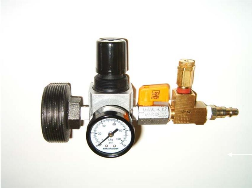
Figure 7: Typical Leak Check Test Fixture
