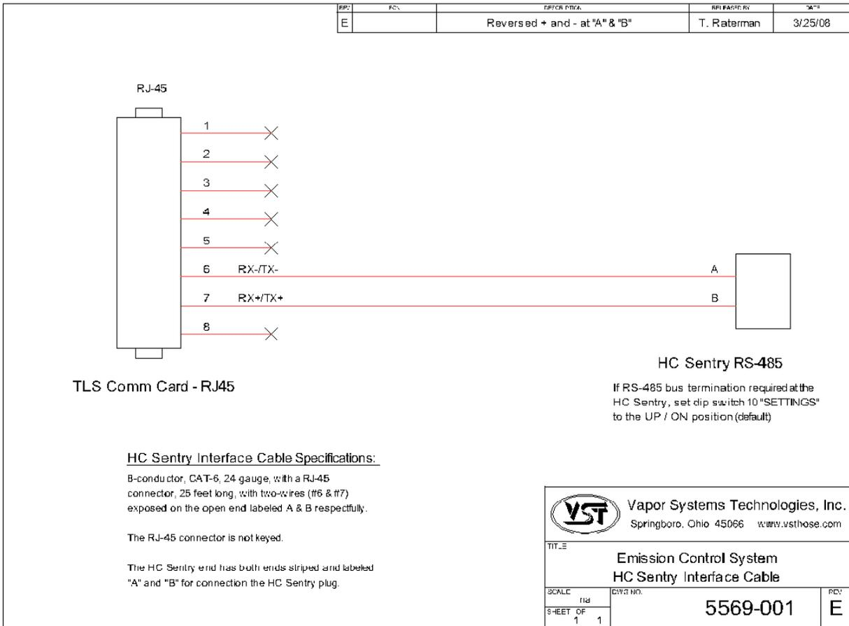
Figure 33: HC Sentry RS-485 Cable Wiring Diagram
