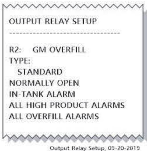
Figure 6-11: Output Relay Setup
