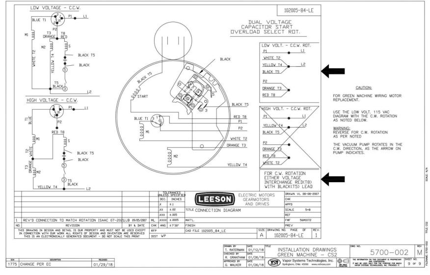
Figure 6-5: Vacuum Pump Motor Wiring Diagram
