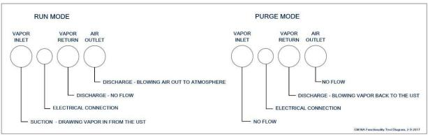
Figure 6-10: GREEN MACHINE Operation Diagram
