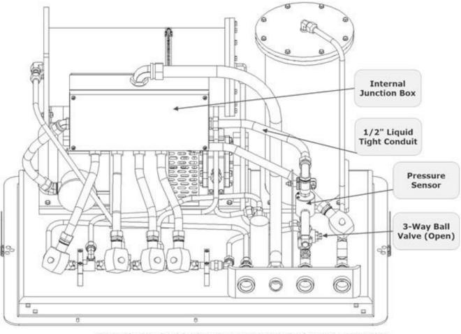
Green Machine Dual Canister Pressure Sensor Replacement, 09-23-2019
