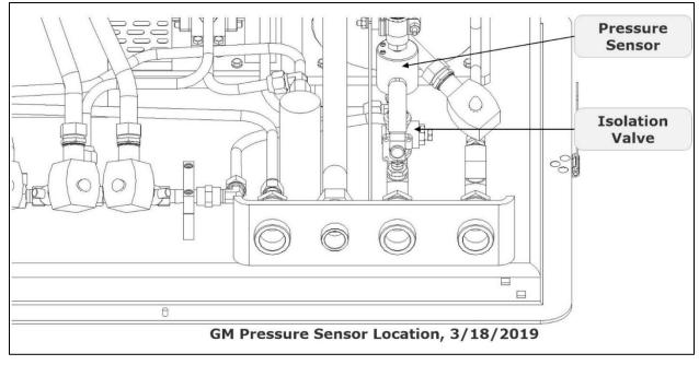
Figure 2-3: Pressure Sensor w/ 3-Way Isolation Valve Open
