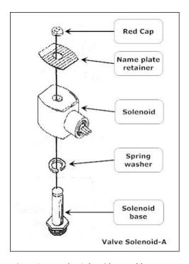
Figure 9-17: Valve Solenoid Assembly
