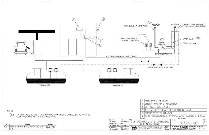
Figure 11-1: GREEN MACHINE Gasoline Station Overview
