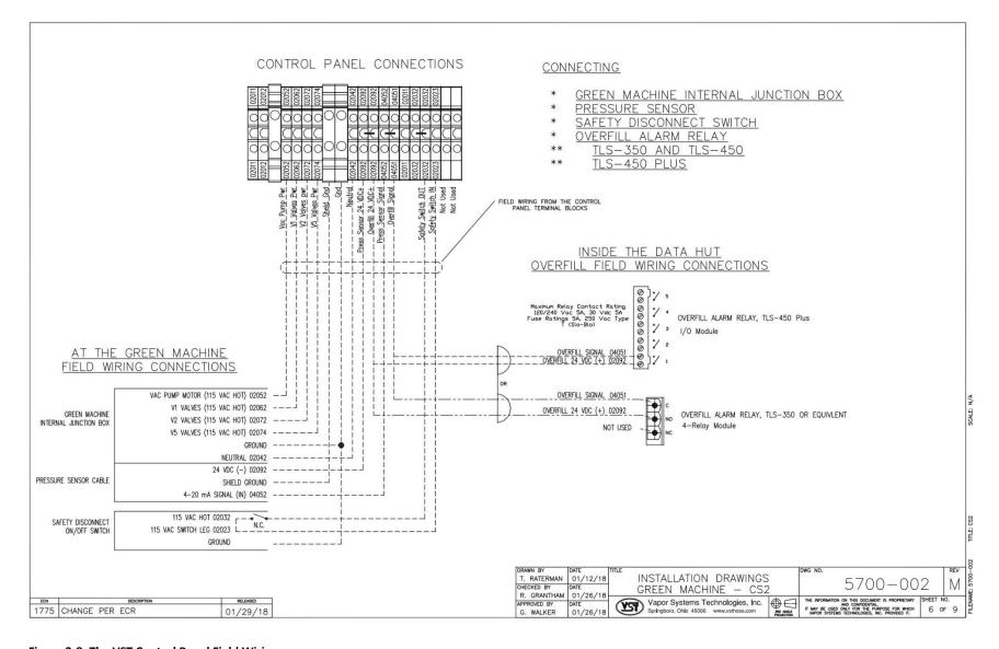
Figure 3-8: The VST Control Panel Field Wiring
