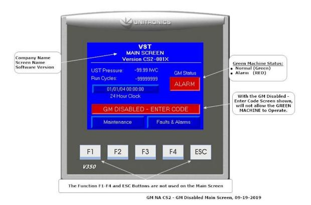
Figure 3-1: Control Panel PLC Main Screen - GM Disabled - Enter CODE Main Screen
