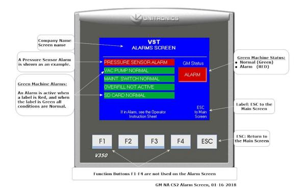
Figure 11-5: Pressure Sensor Alarm shown on the Faults & Alarms Screen
