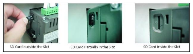
Figure 10-5: Inserting and Removing the SD Card from the PLC
