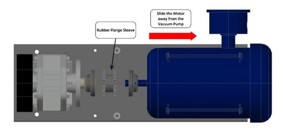
Vacuum Pump Rubber Flange Sleeve Replacement- A1
