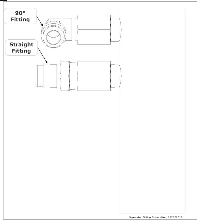
Figure 7-19: Separator Fitting Orientation
