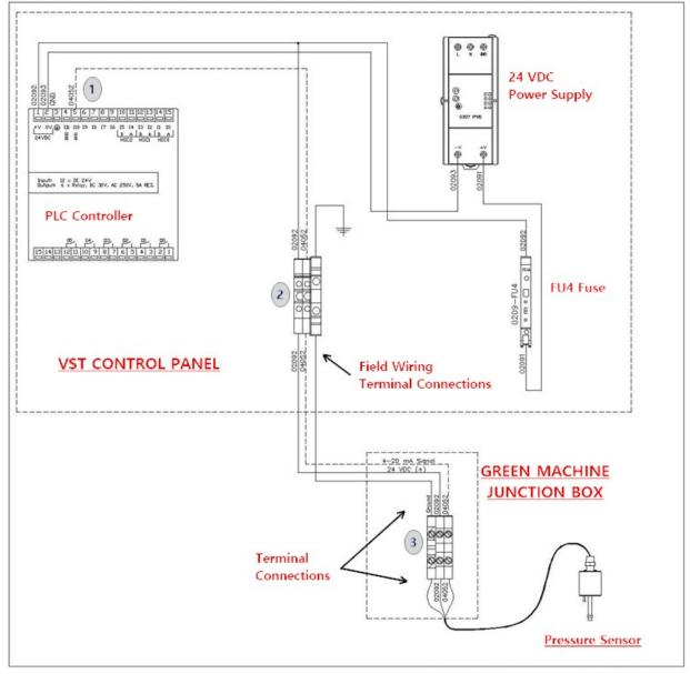
Pressure Sensor Wiring Diagram, 3-5-2019
