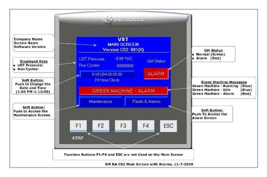
Figure 8-2: VST GREEN MACHINE Control Panel Main Screen with an Alarm Active
