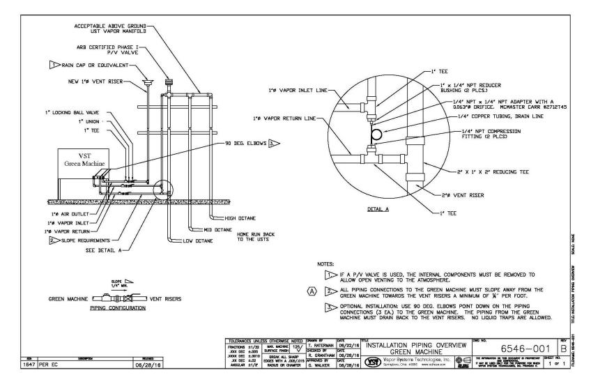
Figure 6-7: GREEN MACHINE Vapor Piping Layout
