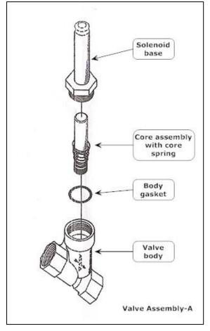
Figure 7-16: Valve Core Assembly
