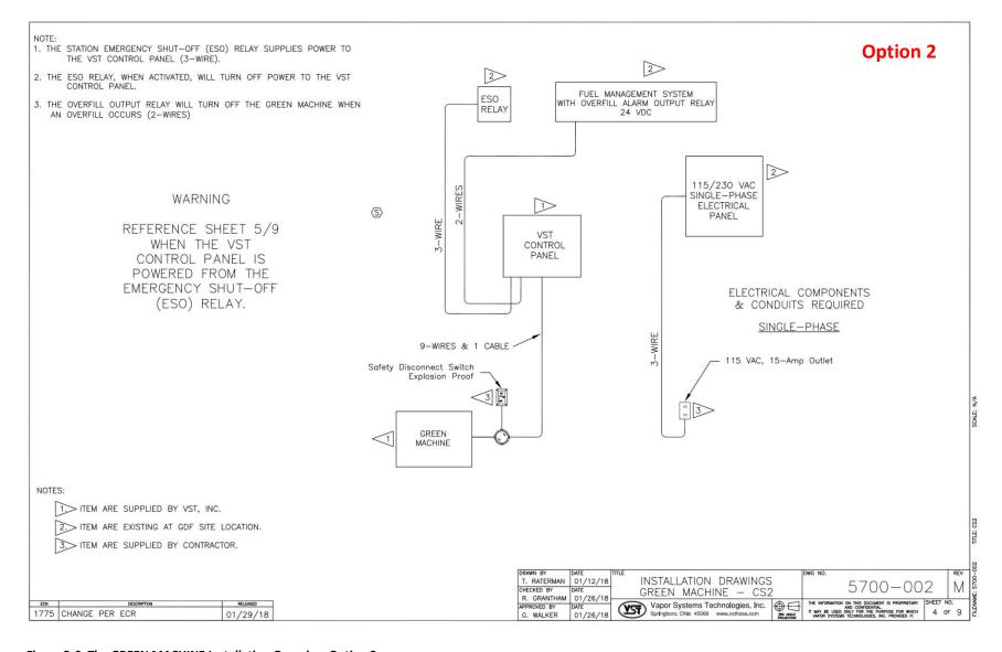
Figure 3-6: The GREEN MACHINE Installation Overview Option 2
