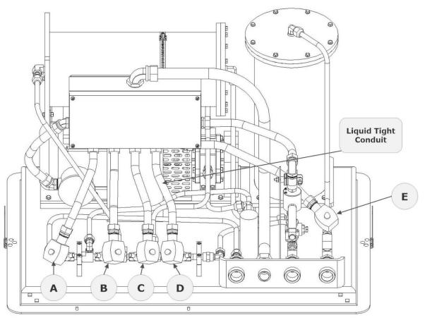
GM Dual Canister Control Valve Replacement Diagram, 09-20-2019
