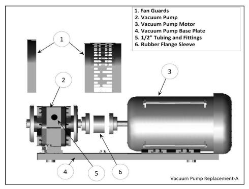
Figure 9-19: Vacuum Pump Components
