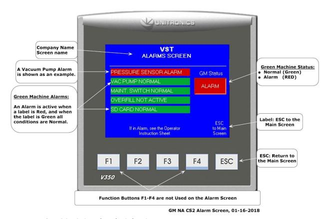
Figure 3-2: VST Control Panel PLC Alarm Screen
