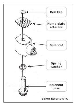
Figure 7-14: Valve Solenoid Assembly
