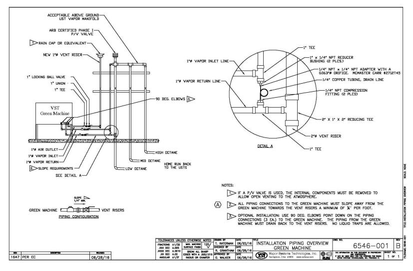
Figure 7-4: GREEN MACHINE Vapor Piping Layout
