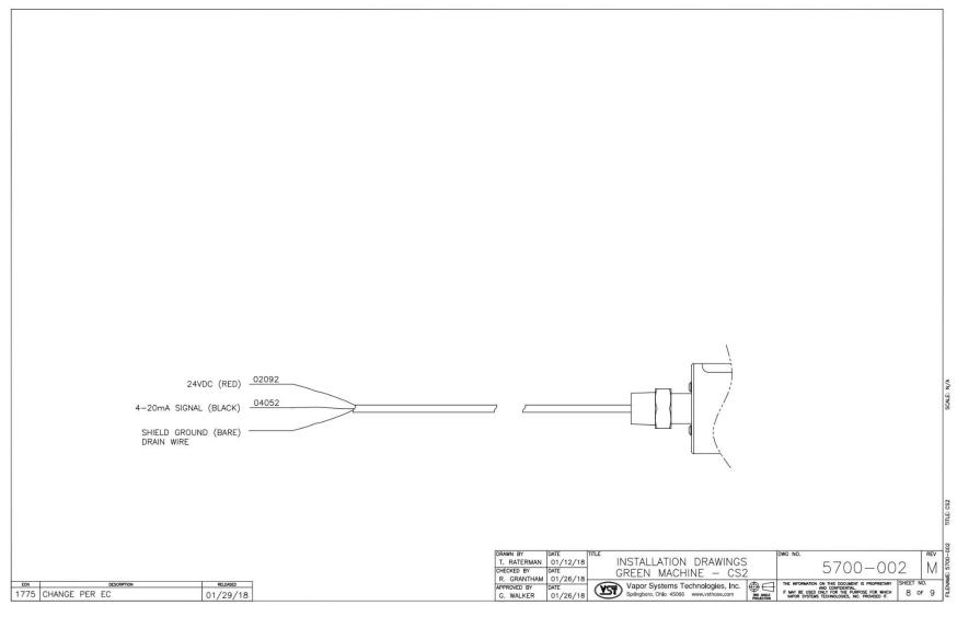
Figure 3-10: Pressure Sensor Wiring Diagram
