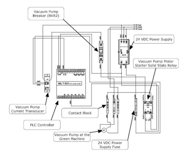
Vacuum Pump Power and Control Circuit, 3-9-2018
