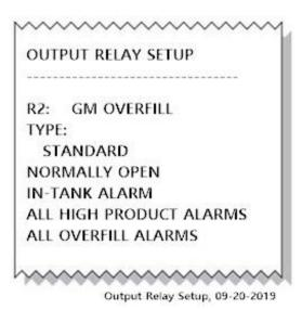
Figure 6-11: Output Relay Setup
