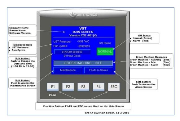
Figure 8-1: VST GREEN MACHINE Control Panel Main Screen
