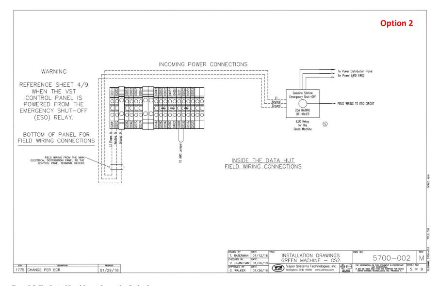
Figure 3-7: The Control Panel Power Connection Option 2
