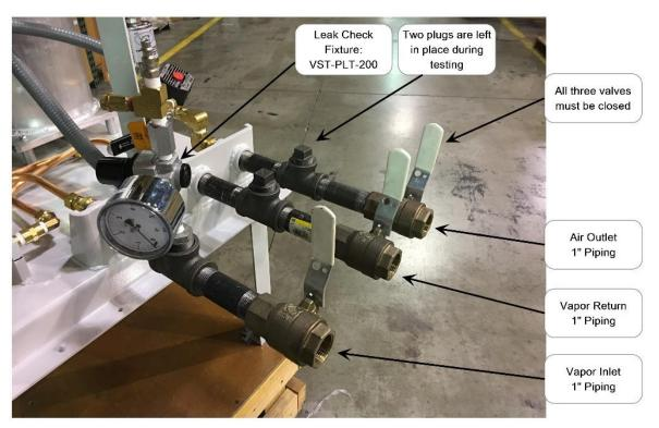
GM Leak Check Test Fixture-B, 11-2-2016
