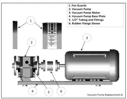
Figure 9-14: Vacuum Pump Components
