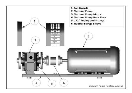
Figure 9-22: Vacuum Pump Assembly and Components
