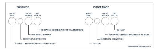
Figure 7-7: GREEN MACHINE Operation Diagram
