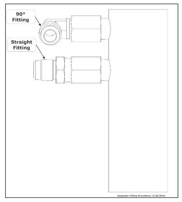
Figure 9-35: Separator Fitting Orientation
