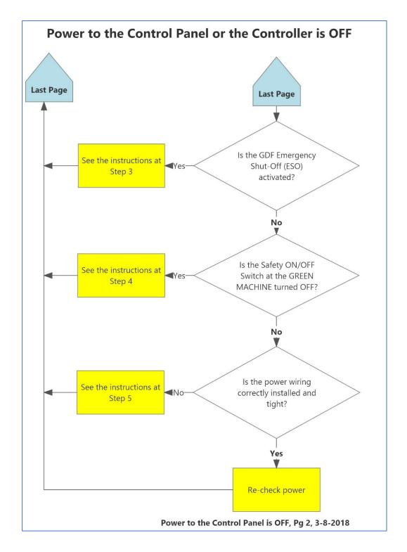
Figure 8-4 continued... Power to the VST Control Panel or Controller is OFF
