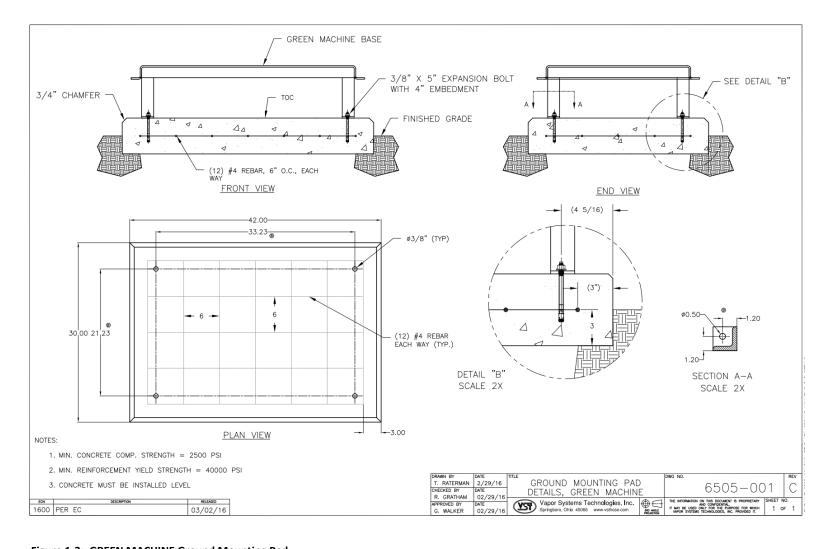
Figure 1-3: GREEN MACHINE Ground Mounting Pad
