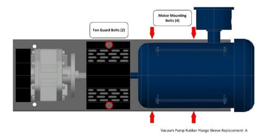
Figure 7-11: Vac Pump Rubber Flange Sleeve Replacement
