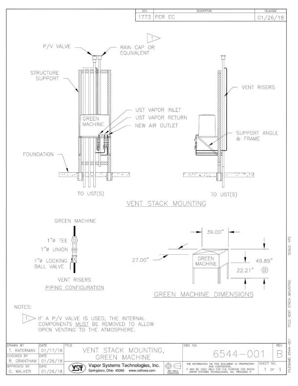
Figure 1-4: Vent Stack Installation
