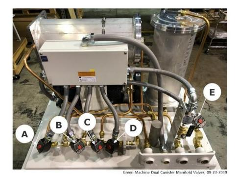
Figure 9-23: Manifold Valves
