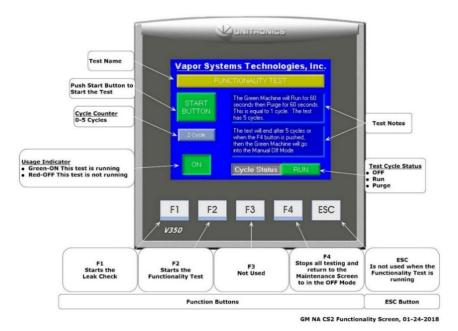
Figure 7-5: Functionality Test Screen
