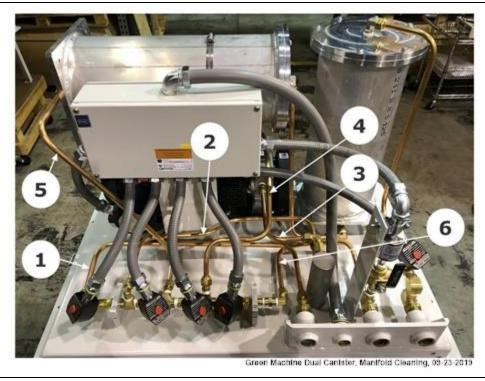
Figure 9-20: Items Associated with Cleaning the GREEN MACHINE Tubing and Manifold
