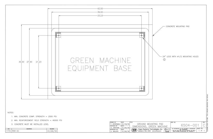
Figure 1-2: Concrete mounting pad dimensions
