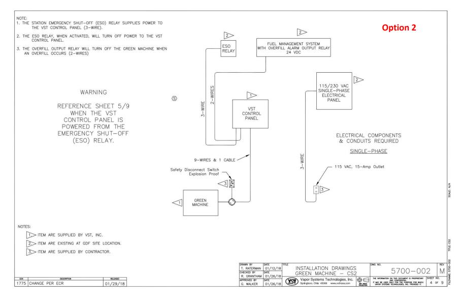
Figure 8-7: VST Control Panel Powered from ESO Relay
