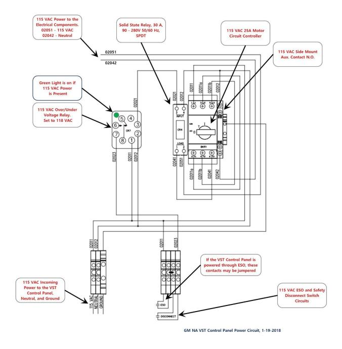
Figure 8-10: VST Control Panel 115 VAC Power Circuit Diagram
