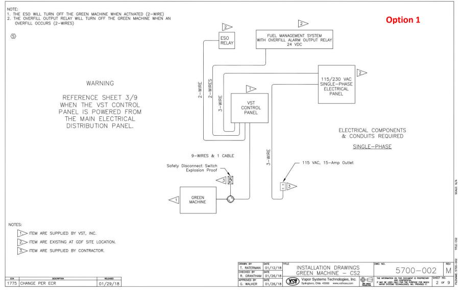
Figure 8-5: Electrical Field Wiring Diagram
