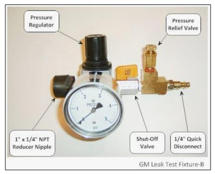
Figure 9-40: Leak Check Fixture
