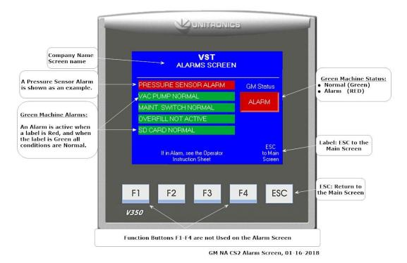
Figure 10-3: Faults & Alarm Screen
