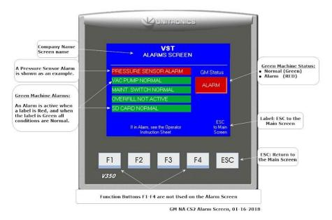
Figure 8-17: GREEN MACHINE Controller Alarm Screen
