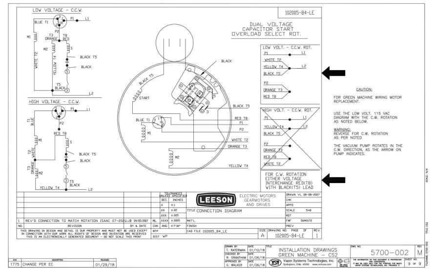
Figure 3-11: Vacuum Pump Motor Wiring Diagram
