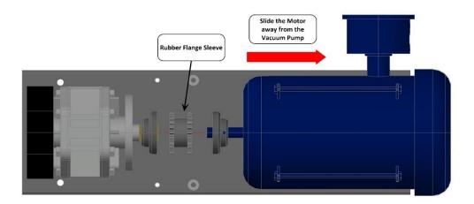
Vacuum Pump Rubber Flange Sleeve Replacement- A1
