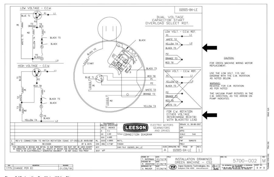
Figure 9-15: Junction Box Motor Wiring Diagram
