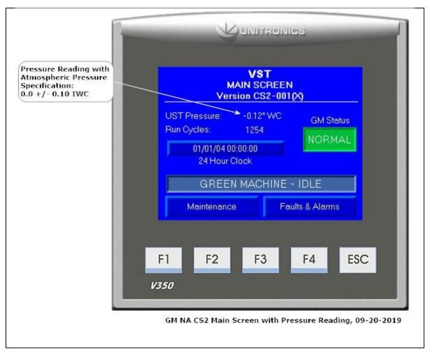
Figure 7-10: Main Screen w/Pressure Reading
