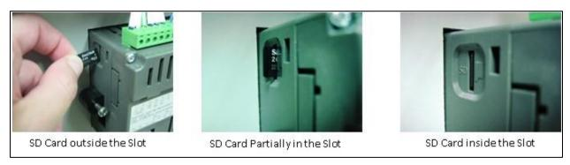
Figure 11-6: Inserting and Removing the SD Card from the PLC
