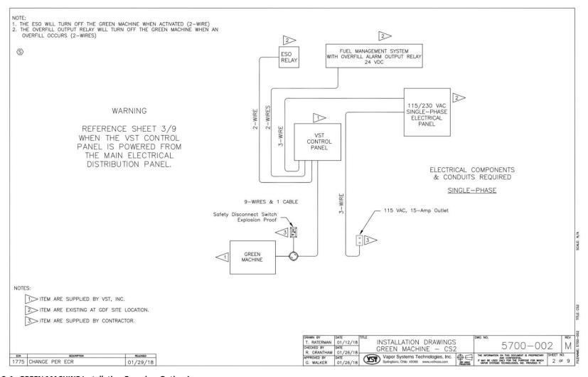
Figure 3-4: GREEN MACHINE Installation Overview Option 1
