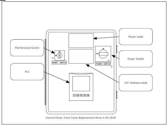
Figure 8-9: VST Control Panel Components – Front Cover
