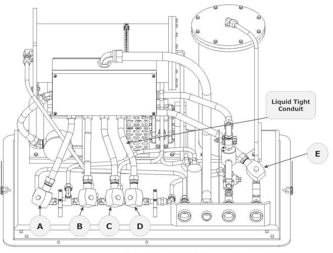
GM Dual Canister Control Valve Replacement Diagram, 09-20-2019
