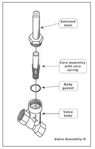
Figure 9-18: Valve Assembly
