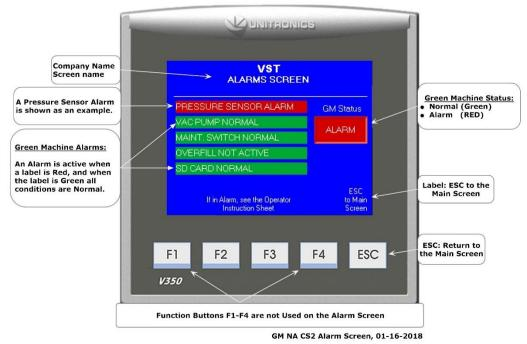
Figure 4-4: Pressure Sensor Alarm shown on the Alarm Screen
