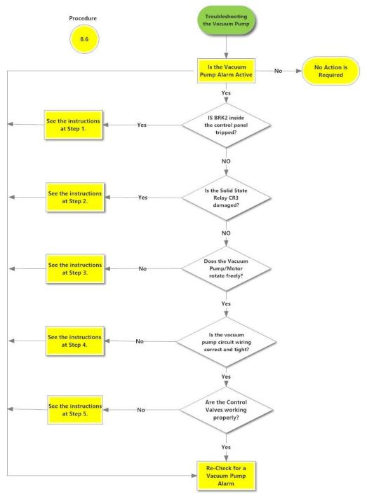
Vacuum Pump Motor Alarm, 3-8-2018
