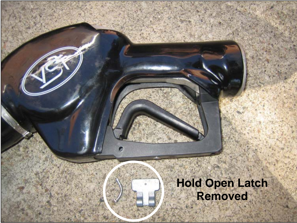
Figure 1 VST Balance Nozzle with Hold Open Latch Removed
