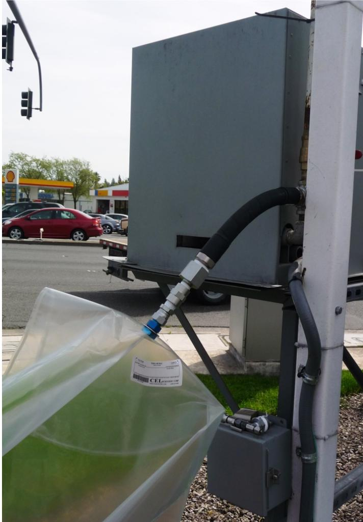
**Figure 10: Tedlar Bag attached to Green Machine**
