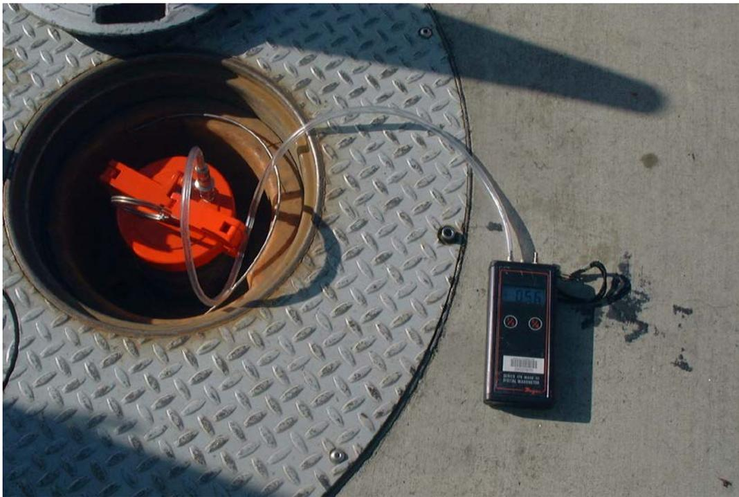
Figure 2 – Vapor Pressure Sensor Test Port
