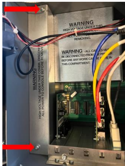
Figure 3-7: Communication Bay Panel Screws
