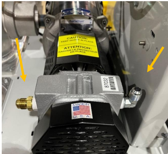
Figure 7-8: Two tubes removed from vacuum pump
