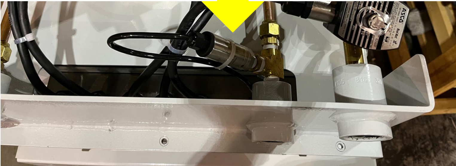
Figure 9-6: Pressure Sensor Installed in GREEN MACHINE
