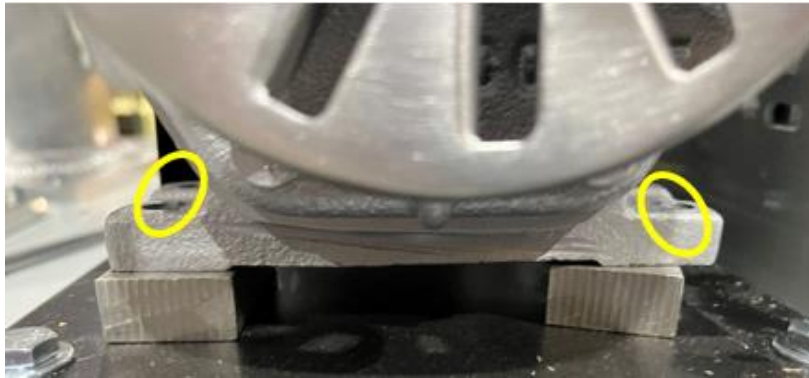
Figure 9-17: Vacuum Pump Mounting Bolts
