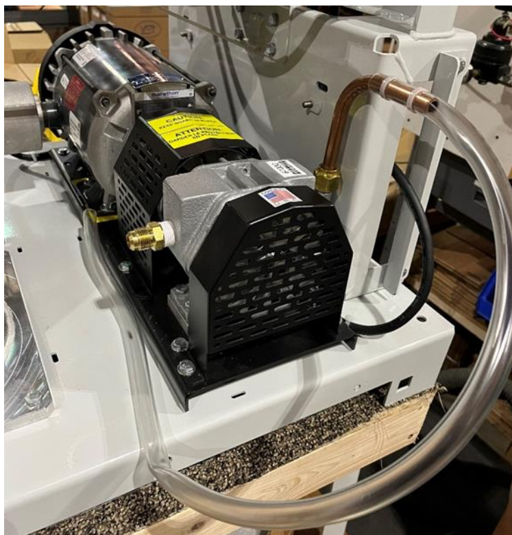
Figure 9-23: Vacuum Pump with the Blowout tube
