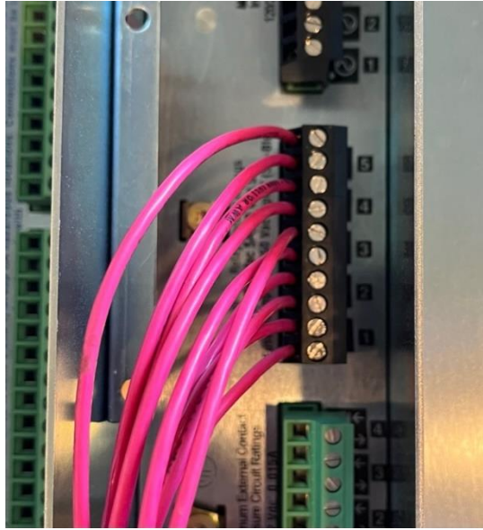
Figure 3-4: No relays available in I/O module
