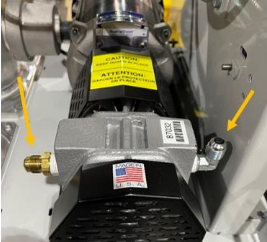
Figure 9-15: Two Tubes Removed from Vacuum Pump
