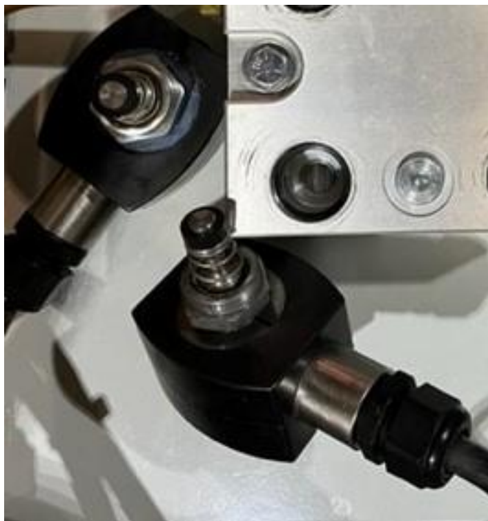
Figure 9-22: Solenoids with the Core Assembly Inside
