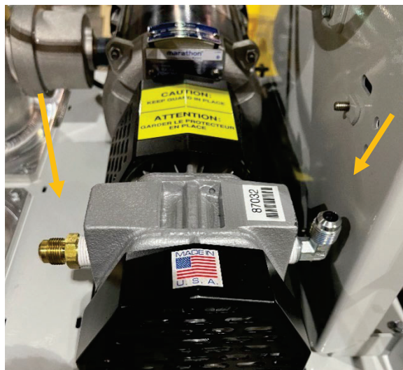
Figure 9-7: Two tubes removed from vacuum pump
