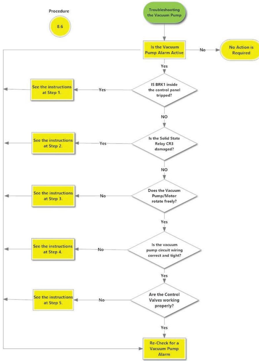
Vacuum Pump Motor Alarm, 10-6-2021
