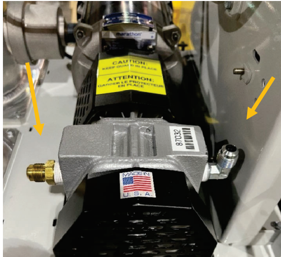
Figure 7-8: Two tubes removed from vacuum pump
