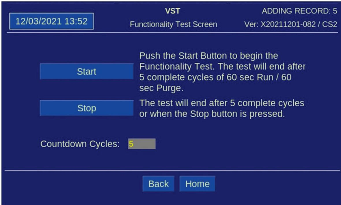
Figure 6-5: Functionality Test Screen
