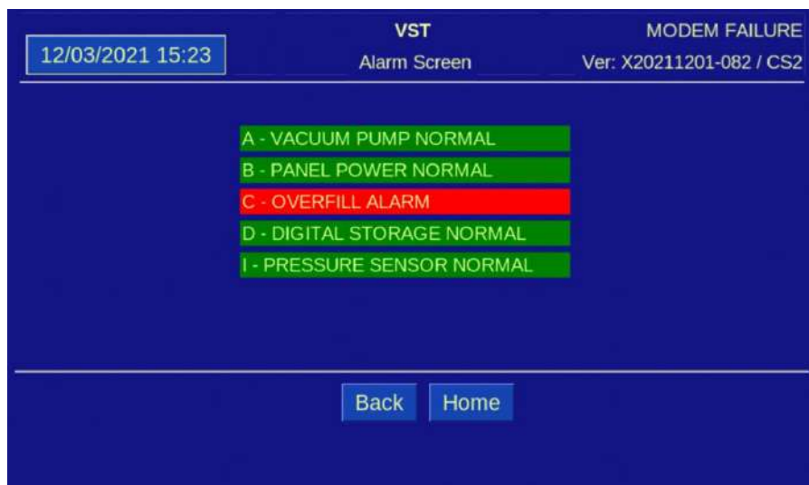
Figure 8-12: GREEN MACHINE PLC Alarm Screen
