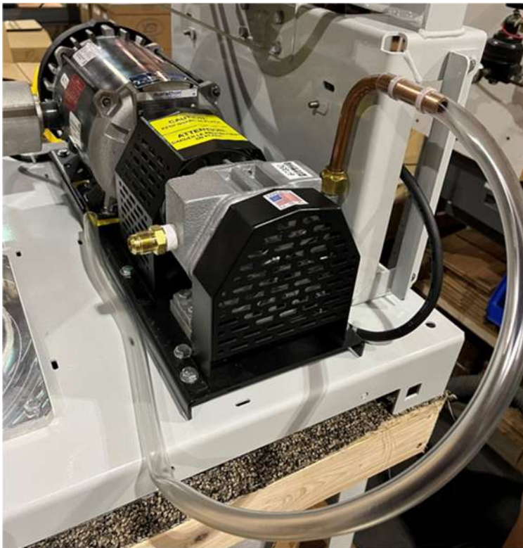
Figure 9-23: Vacuum Pump with the Blowout tube
