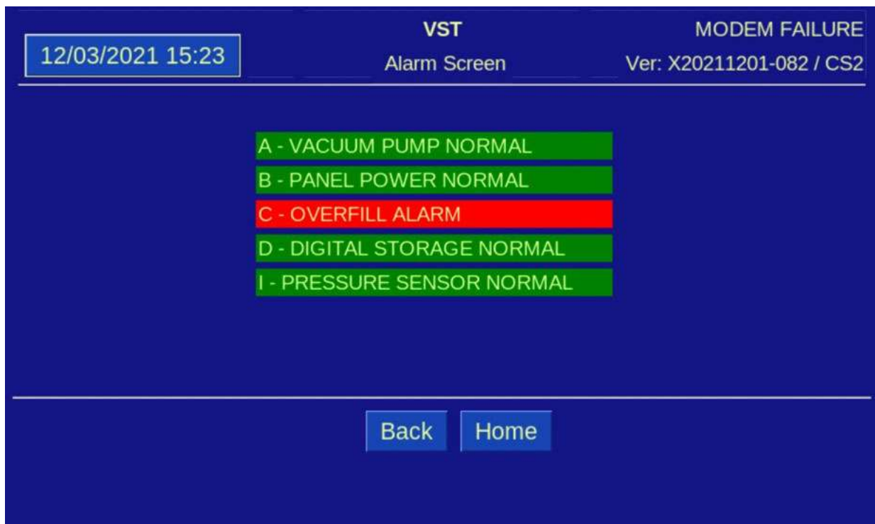
Figure 4-4: Alarm Screen with Active Alarm
