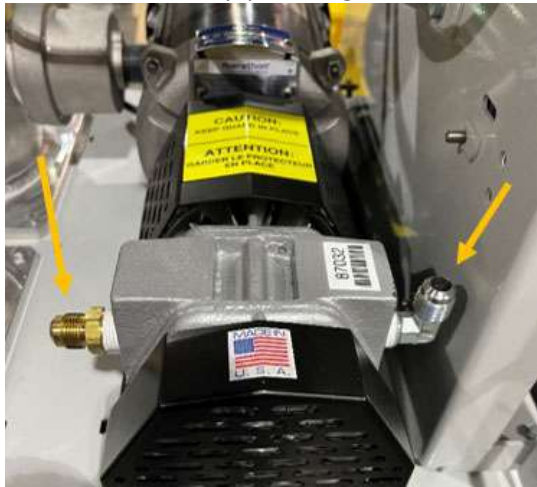
Figure 9-15: Two Tubes Removed from Vacuum Pump
