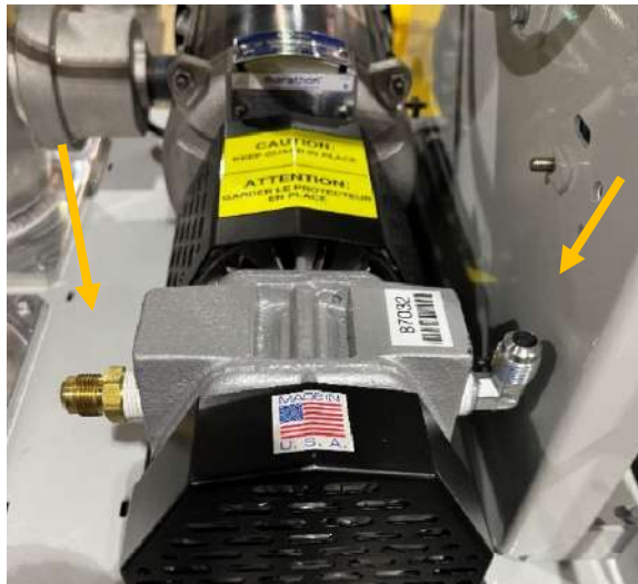
Figure 7-8: Two tubes removed from vacuum pump
