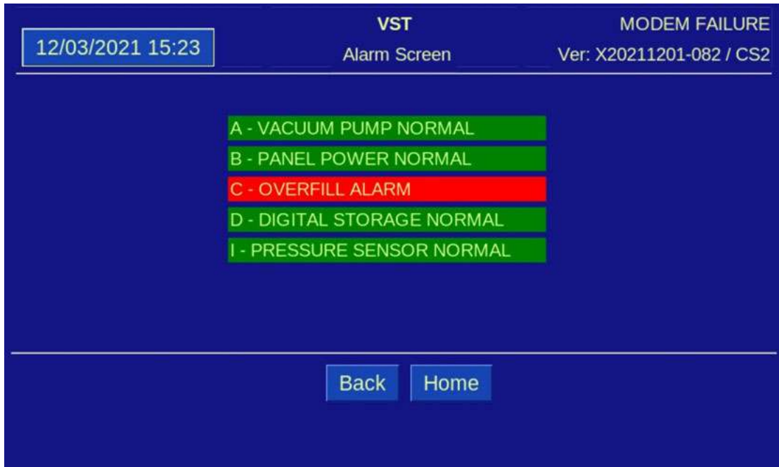
Figure 3-2: VST Control Panel PLC Alarm Screen
