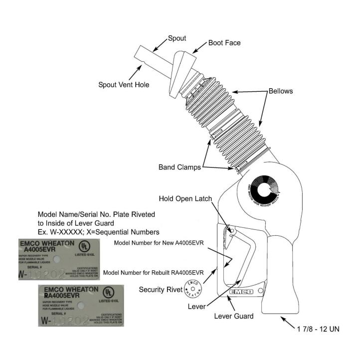
Figure 2B-1 EMCO Model A4005EVR Nozzle
