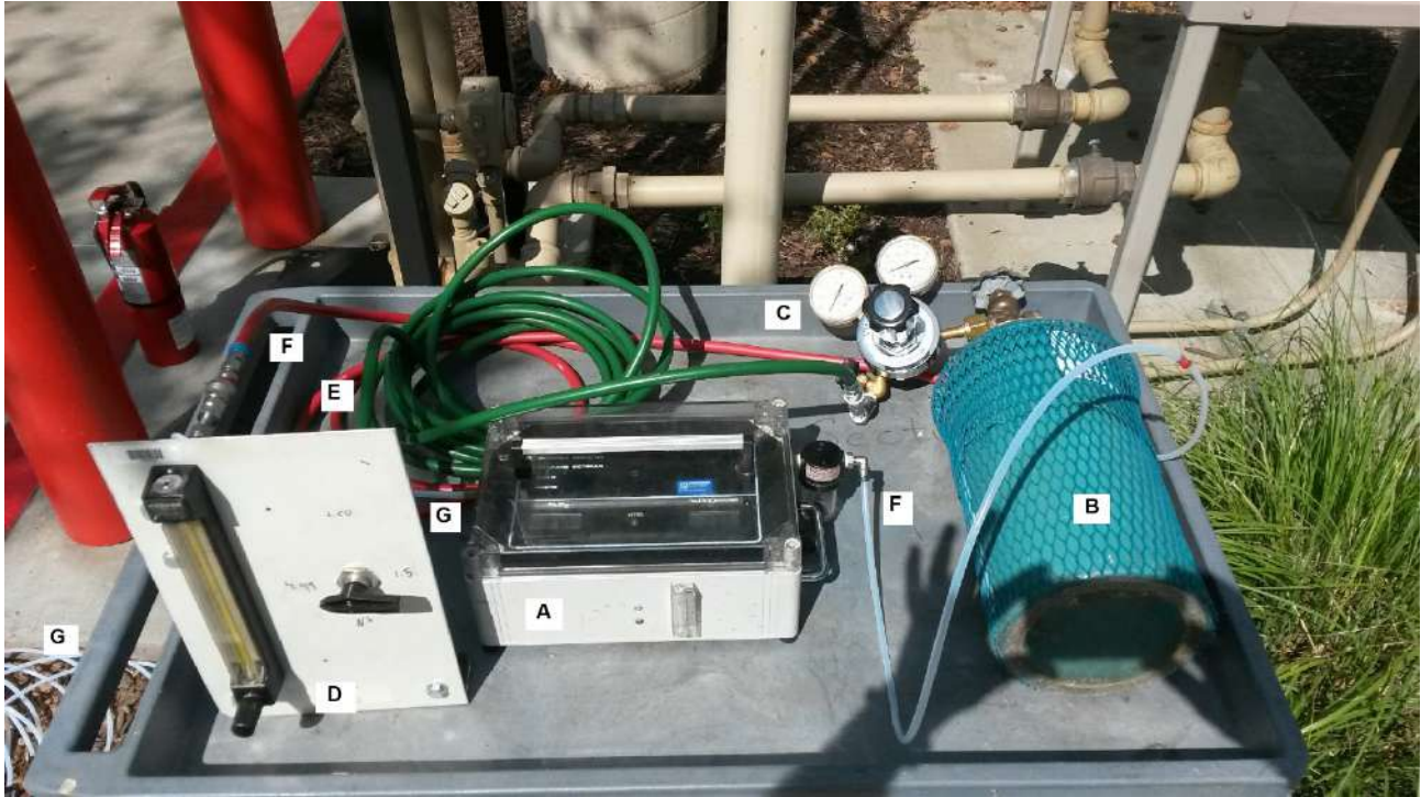
Figure 1 Equipment Configuration for HC Analyzer Calibration
