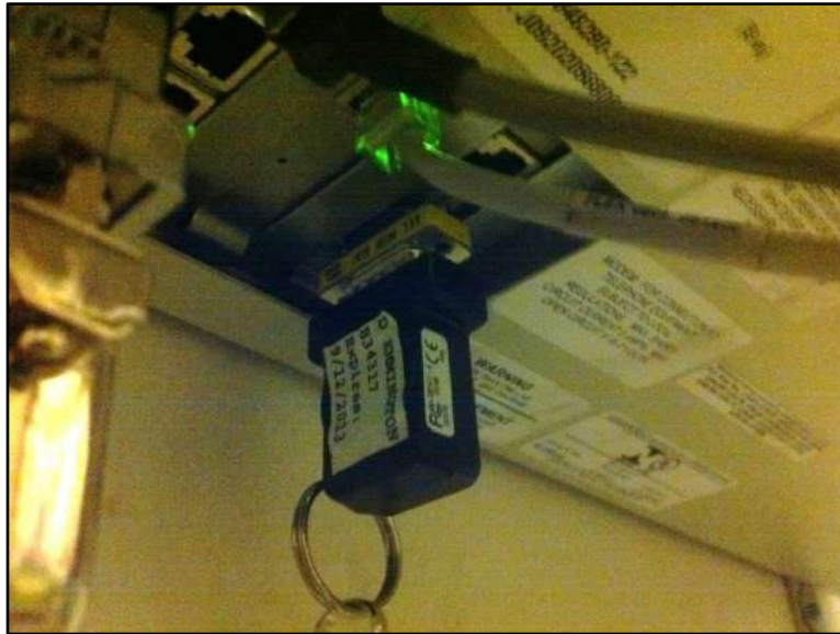
FIGURE 4 Maintenance Tracker Key Plugged Into TLS Console
