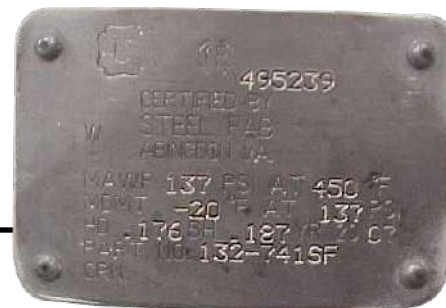
Clean Air Separator Data Plate
