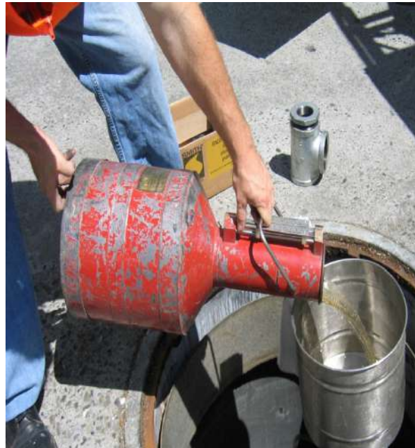
FIGURE 11-3 Adding Gasoline through Open Fuel Entry Point
