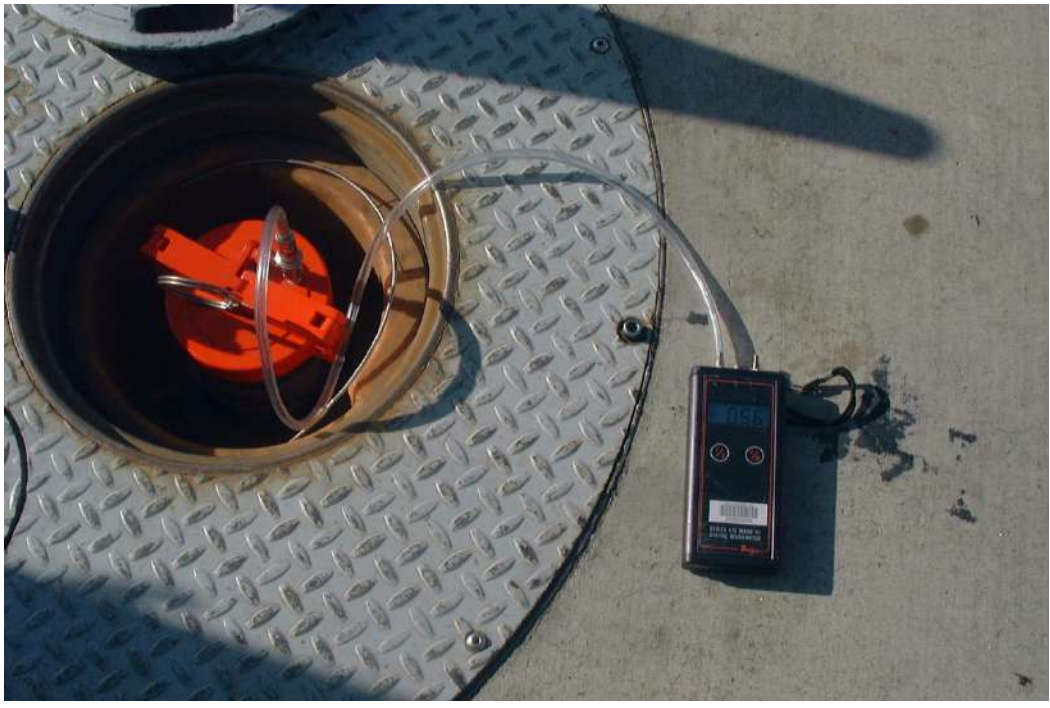
FIGURE 10-1b Typical Field Installation of UST Pressure Measurement Assembly
