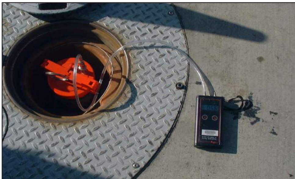
FIGURE 9-2 Typical Field Installation of UST Pressure Measurement Assembly
