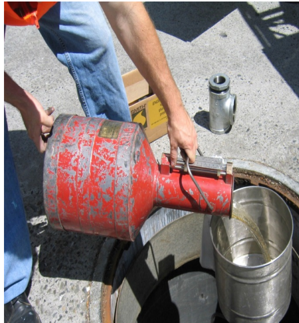
FIGURE 11-3 Adding Gasoline through Open Fuel Entry Point
