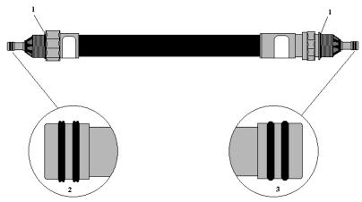
Rule of Thumb: O-rings (item 3) to Nozzle and Hose Adaptor Quad Seals (item 2) to Breakaway (or Flow Limiter)
