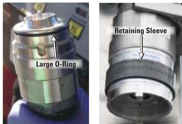
Figure 2: Check each half for damage
