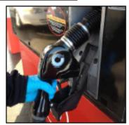
Remove the nozzle from the dispenser cradle without touching the lever. If the hold-open latch is engaged, the nozzle fails. The nozzle shall not be used and must be immediately taken out of service.
