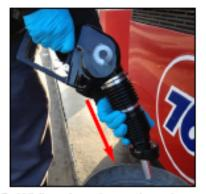
5. While keeping the lever engaged, slowly allow the bellows to extend to its "free" position in a controlled manner that simulates removing the nozzle from a vehicle fill pipe. Make sure that the boot face is not caught on the spout latch ring.
