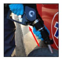
4. While pointing the end of the spout downwards into a gasoline approved container compress the bellows from its "free" extended position, and engage (squeeze) the lever. If the lever exhibits no tension (dead lever), the nozzle fails. The nozzle shall not be used and must be immediately taken out of service.
