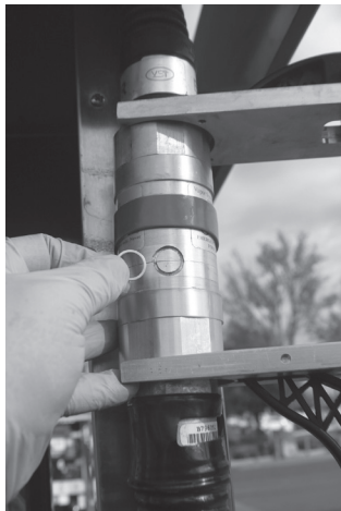
Figure 6: Add Shear Washer Figure 7: Remove Grease
