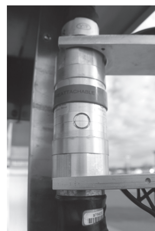
Figure 5: Align Poppet Pin from upper to lower half of breakaway and finish alignment
