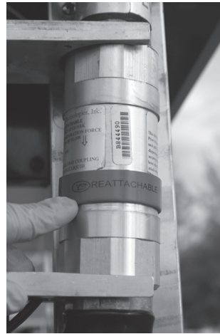
Figure 8: Reposition Retaining Sleeve
