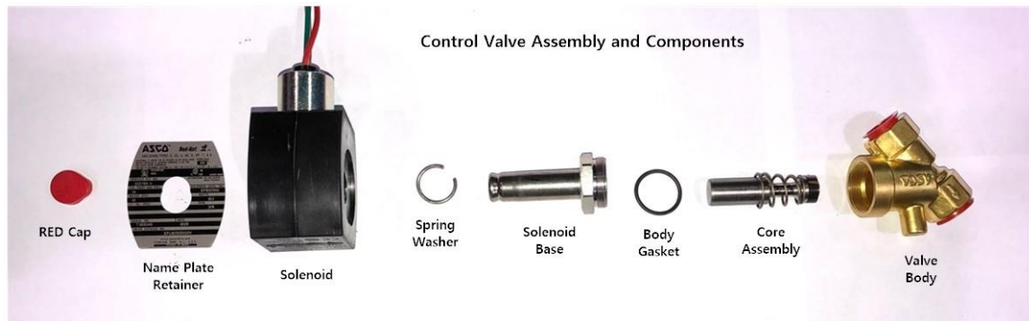
GM Control Valve Assembly and Components, 01-25-2019
