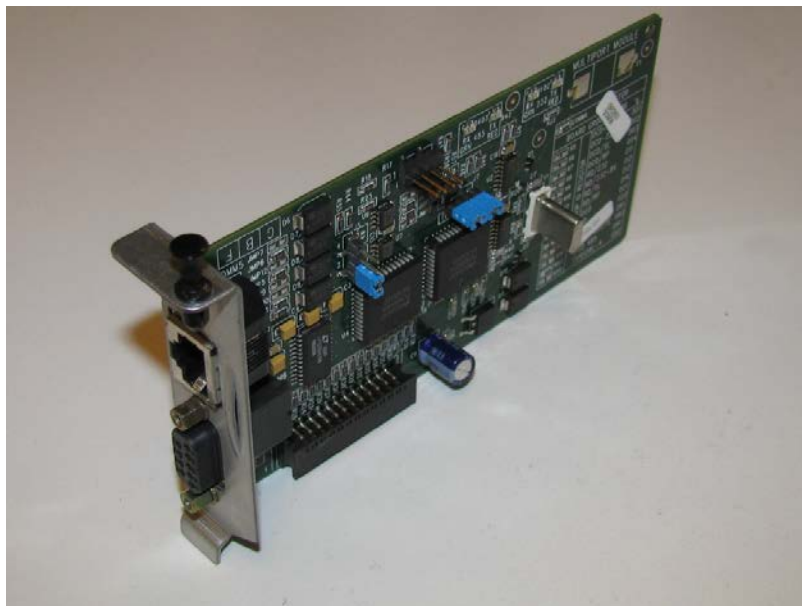
Figure 2B-29 Veeder-Root RS232 Interface Modules Required for Maintenance Tracker
