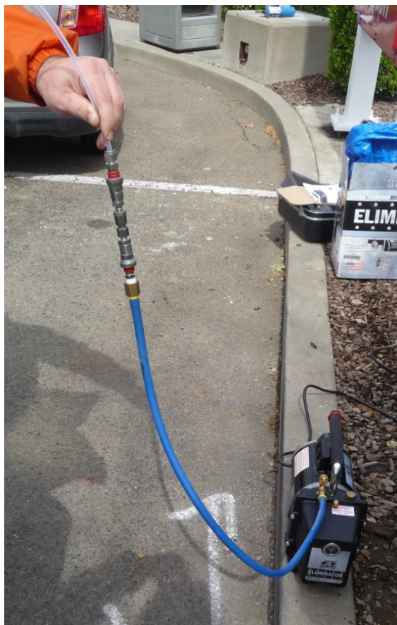
Figure 4: Attach Tedlar Bag to Vacuum Pump to Evacuate the Nitrogen
