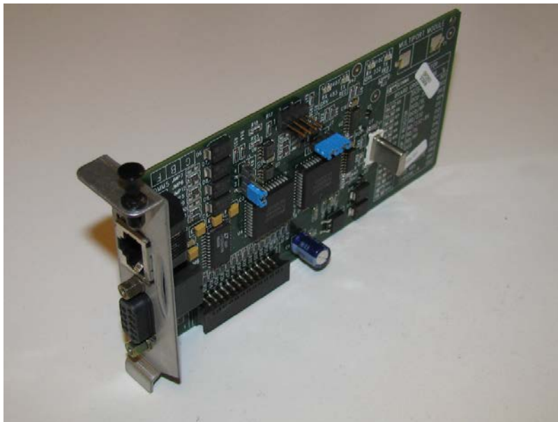
Figure 1A-16 Veeder-Root RS232 Interface Modules Required for Maintenance Tracker
