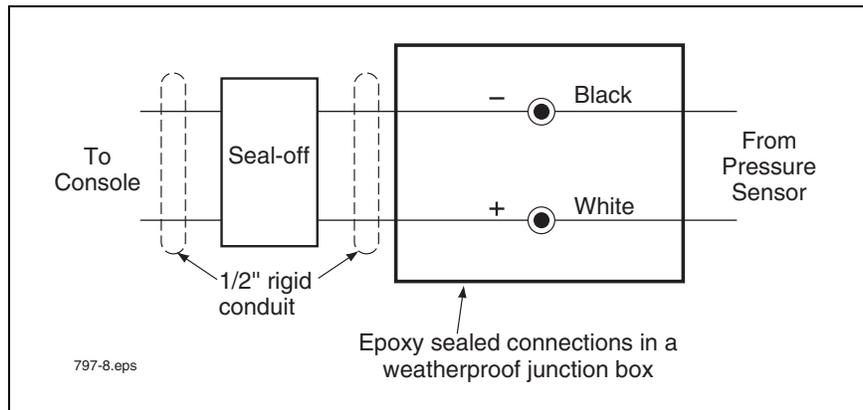
Figure 3. Field wiring Pressure Sensor - Observe Polarity
