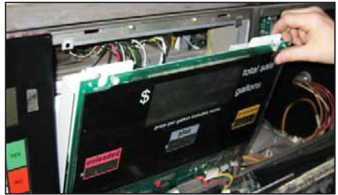
Figure 4: Lower Display Assembly
