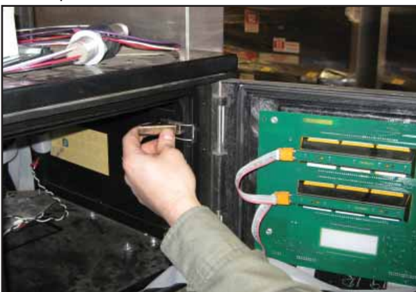
Figure 3: Release Options Door
