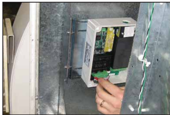
Figure 3: Attach DTU to Dispenser
