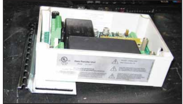
Figure 10: Mounting Bracket on DTU
