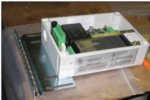
Figure 2: Install Mounting Bracket
