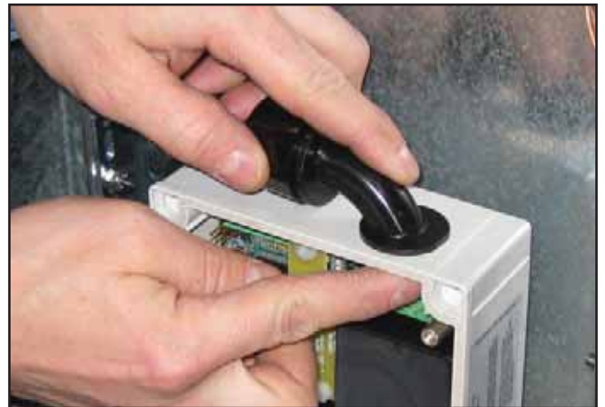
Figure 13: Attach 90-Degree Fitting
