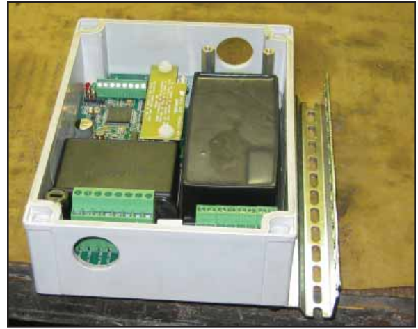
Figure 7: DTU Mounting Bracket Installed
