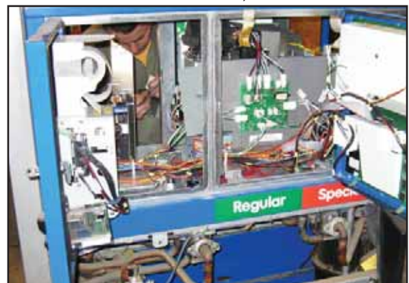
Figure 5: Remove Lower Door
