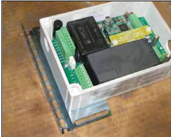
Figure 7: Mounting Bracket on DTU
