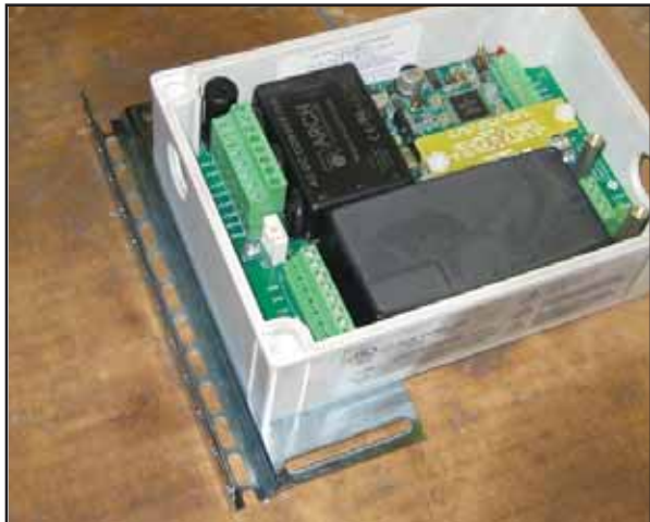
Figure 6: Mounting Bracket on DTU
