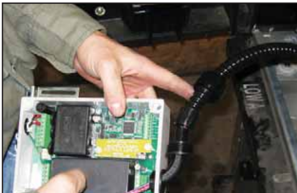
Figure 13: Attach Flexible Conduit to DTU
