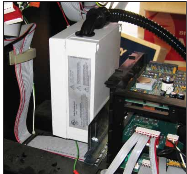
Figure 15: Attach DTU Mounting Bracket
