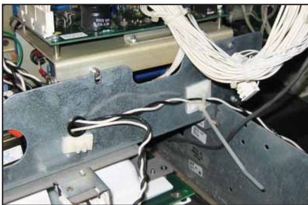
Figure 13: Attach Power Wiring Harness
