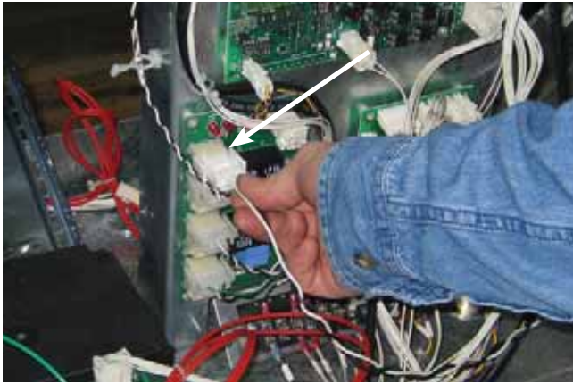
Figure 6: Attach Power Connector to Board
