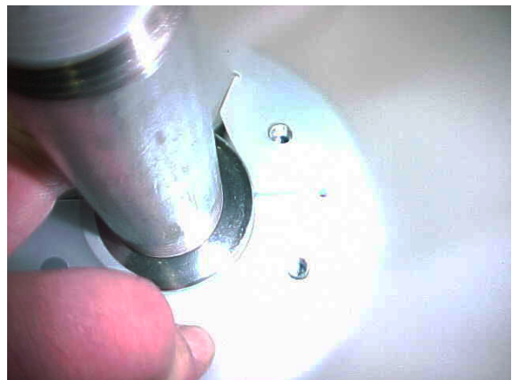
Figure 2: Place Bladder on Flange
