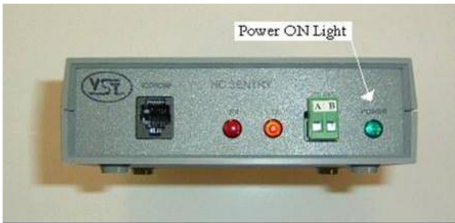
Figure 18: HC Sentry Interface Module Back View: Power "ON" Light
