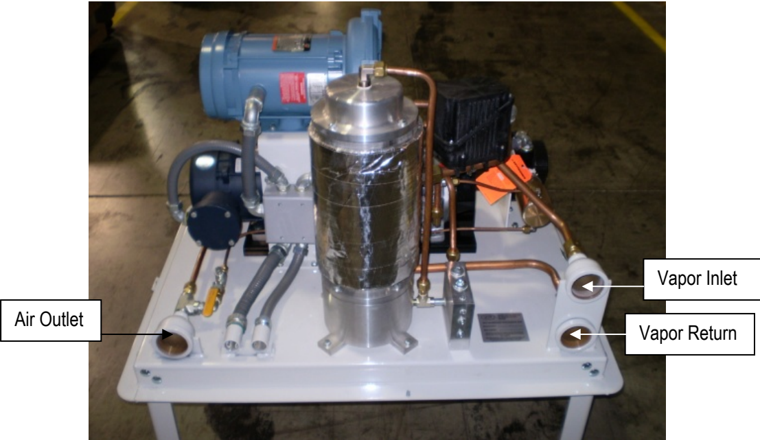
Figure 6: Processor Inlets & Outlets
