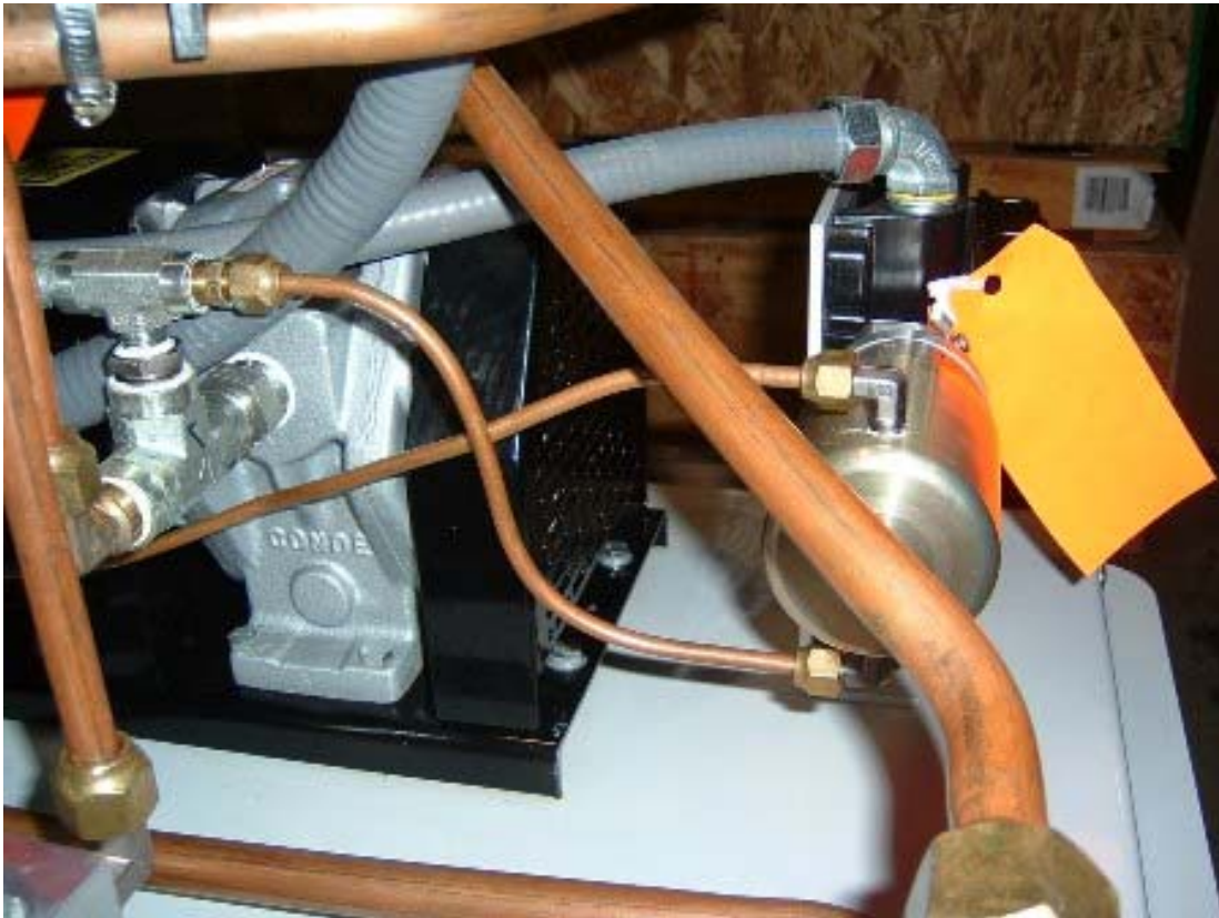
Figure 50: HC IR Sensor Module 1/4" 45° tubing and fittings
