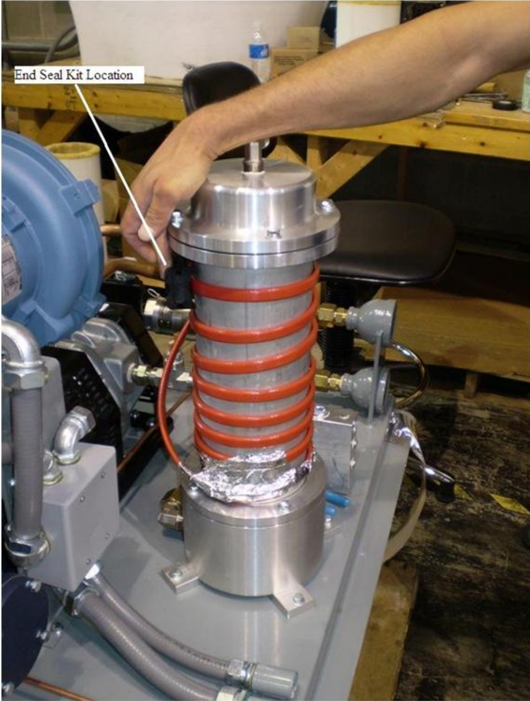
Figure 47: End seal kit location and heat trace cable installation
