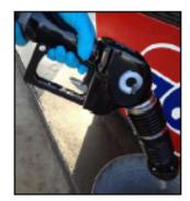
Point the end of the spout downwards into a gasoline approval container. Engage (squeeze) the lever without compressing the bellows. Perform this step a minimum of three times to assure the lever has free motion and no tension (dead lever). IMPORTANT: If at any time while performing step 2 the lever exhibits tension (live lever), the nozzle fails. The nozzle shall not be used and must be immediately taken out of service.
