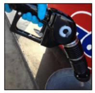
While pointing the end of the spout downwards into a gasoline approved container, engage (squeeze) the lever without compressing the bellows. Perform this step a minimum of three times to assure the lever has free motion and no tension (dead lever).
