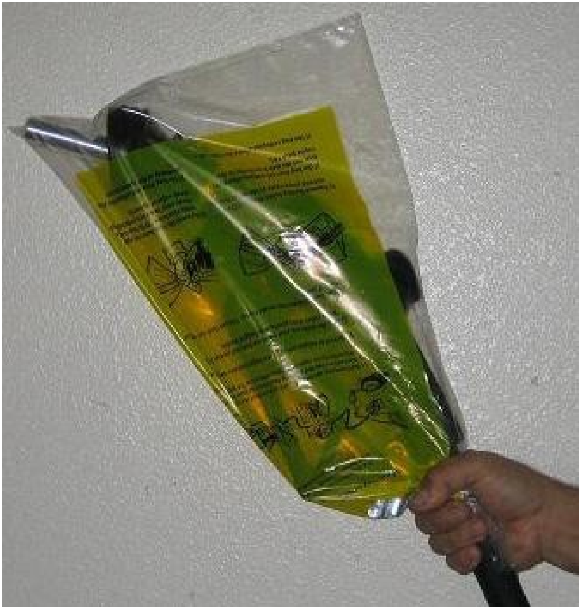
FIGURE 7-1 Typical Example of Bagging a Nozzle
