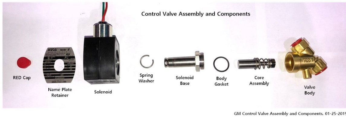
Figure 9-24: GM Control Valve Assembly and Components
