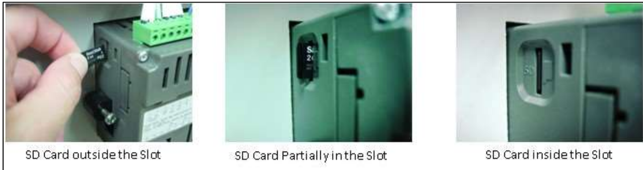
Figure 11-6: Inserting and Removing the SD Card from the PLC
