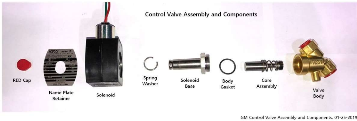
Figure 9-24: GM Control Valve Assembly and Components
