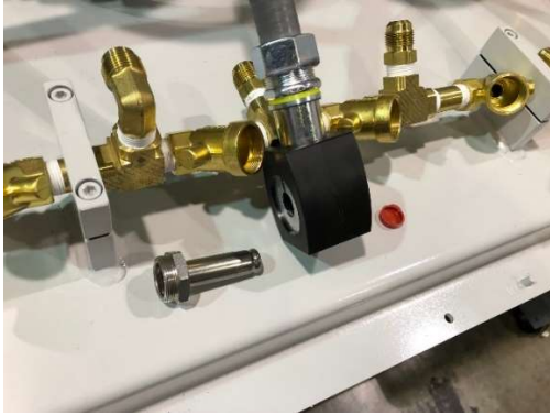
Figure 9-27: Solenoid with Solenoid Base and RED Cap
