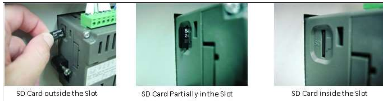
Figure 10-5: Inserting and Removing the SD Card from the PLC
