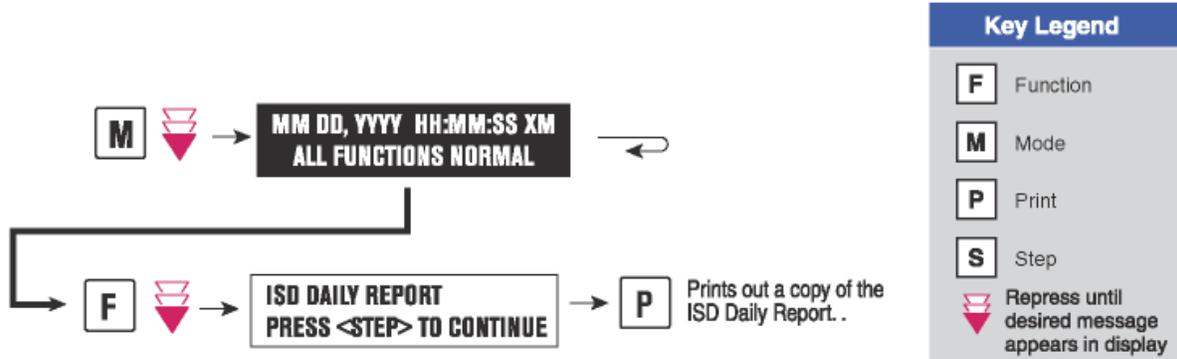
The ISD version number can be verified on the TLS Console LCD screen using the <STEP> key or by using the TLS Console <PRINT> key to print and review the latest ISD Daily Report:
