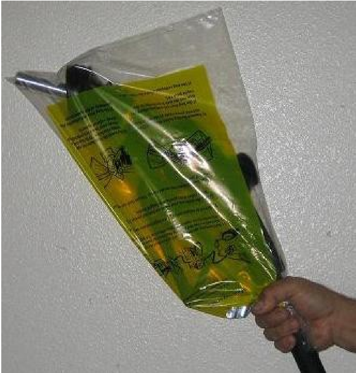
FIGURE 7-1 Typical Example of Bagging a Nozzle
