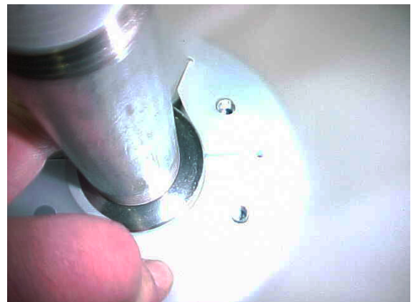
Figure 2: Place Bladder on Flange
