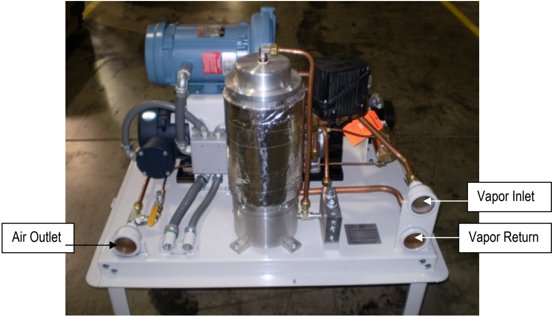
Figure 19: Processor Inlets & Outlets
