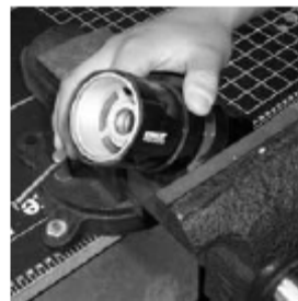
A4119EVR Safe Break Valve
