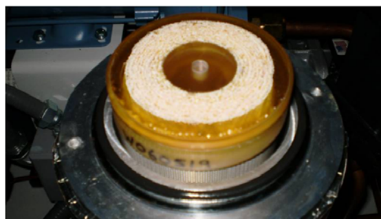
Figure 30: Exposed membrane with top plate removed.
