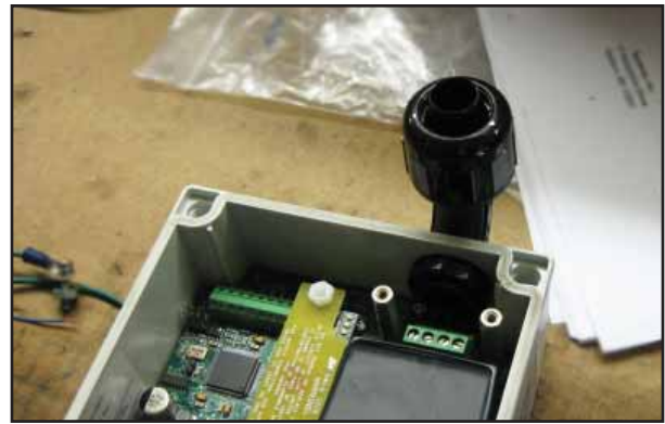
Figure 8: 90-Degree Fitting Installed
